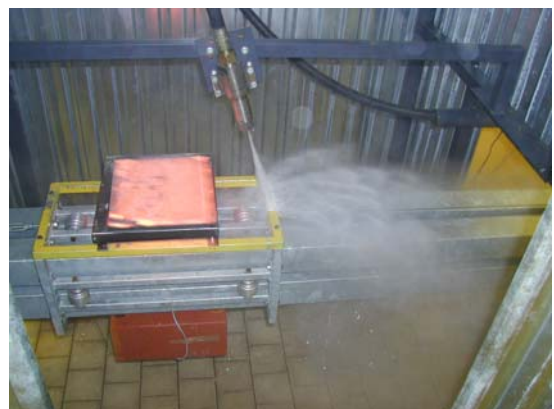
Photo 2 – Test plate moving under the descaling nozzle
