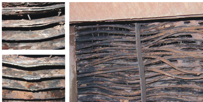
Figure 3 Heat exchanger after operation (Courtesy of EVECO Brno Ltd)
