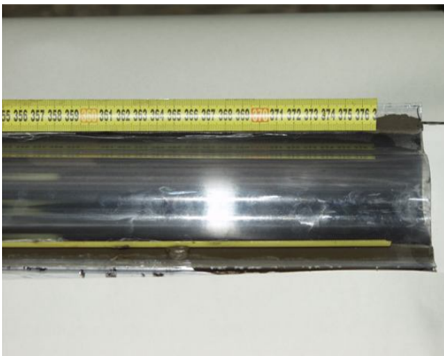
Figure 16. Plastic corrugated tube (i.e. \theta=0 ) to measure, by PIV-method, velocity profiles (see Table 1)
