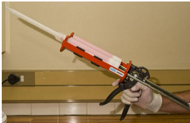
Figure 15 Cartridge inserted into handgun.
