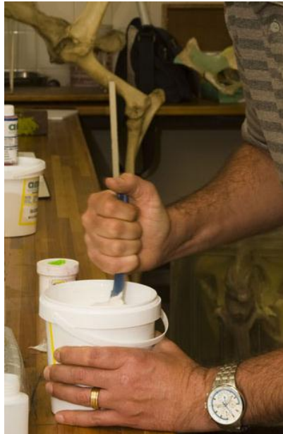
Figure 2 Add thinner to silicone and stir thoroughly for 5 minutes.
