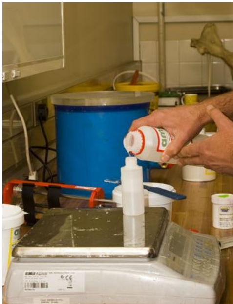
Figure 1 Weigh 10% silicone thinning fluid.
