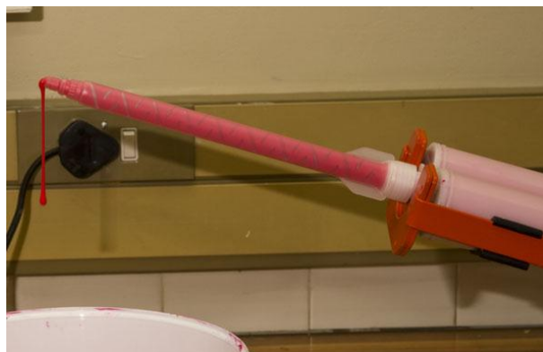
Figure 16 Static mixing nozzle primed.
