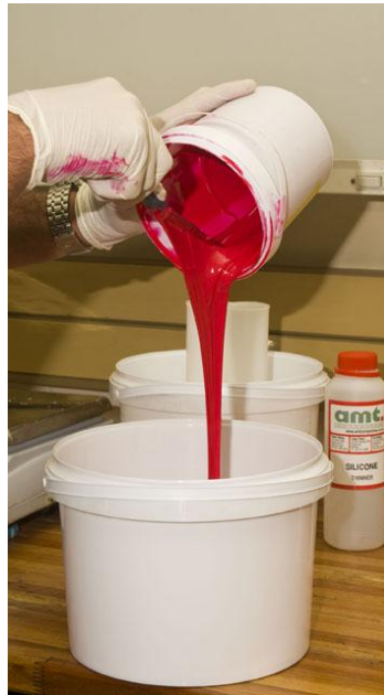
Figure 6 Silicone preparation into a 5 litre bucket.
