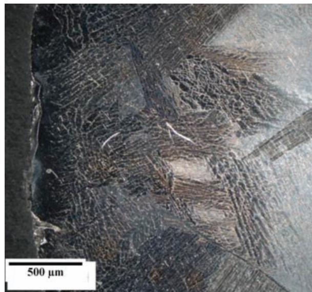
Figure 1 – Alpha case layer after investment casting of Ti-6Al-4V alloy (Mutombo and Rossouw, 2011)
