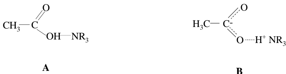
Scheme II: Schematic presentation of (A) molecular and (B) ionic amine-carboxylic acid ( A_1C_1 ) complex (Tamada & King, 1990)
