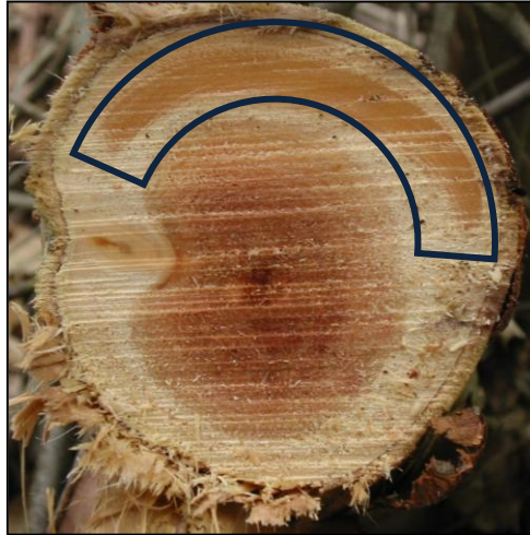
Figure 1.1: Cross section of a Eucalyptus grandis x Eucalyptus urophylla two-year-old stem after prolonged bending showing the visible difference between tension wood (highlighted) and opposite wood (lower-side). (Photo by Forest and Molecular Genetics Programme, University of Pretoria).
