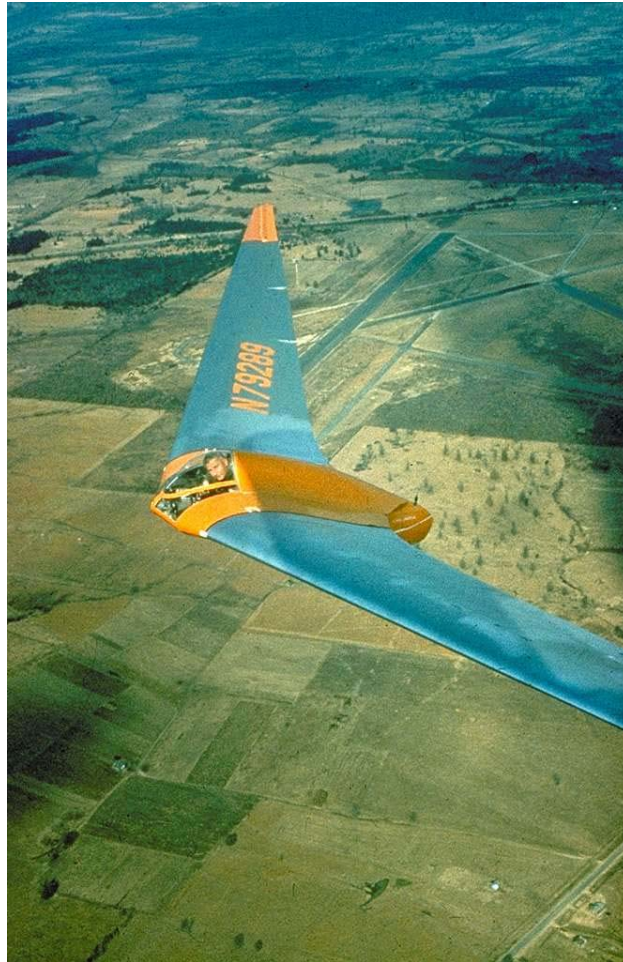
Figure 2.18: The Horten Ho IV flying wing with the pilot in the prone position (RFRL)
