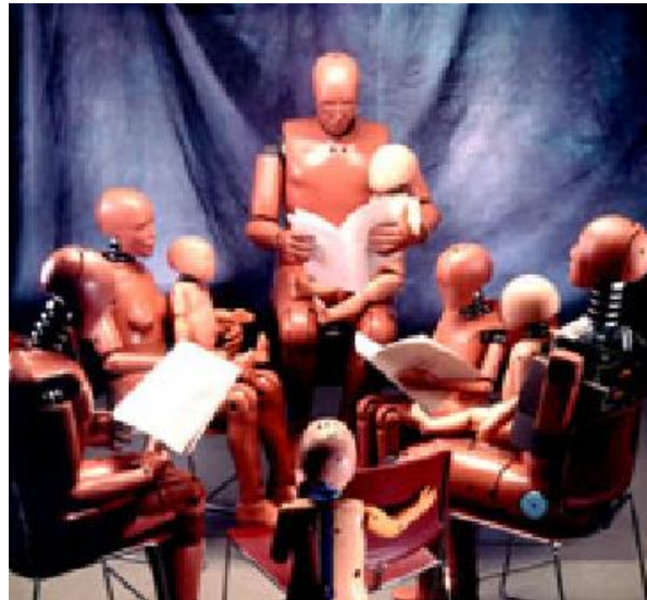
Figure A1. The Hybrid III crash test dummy family (GM)
