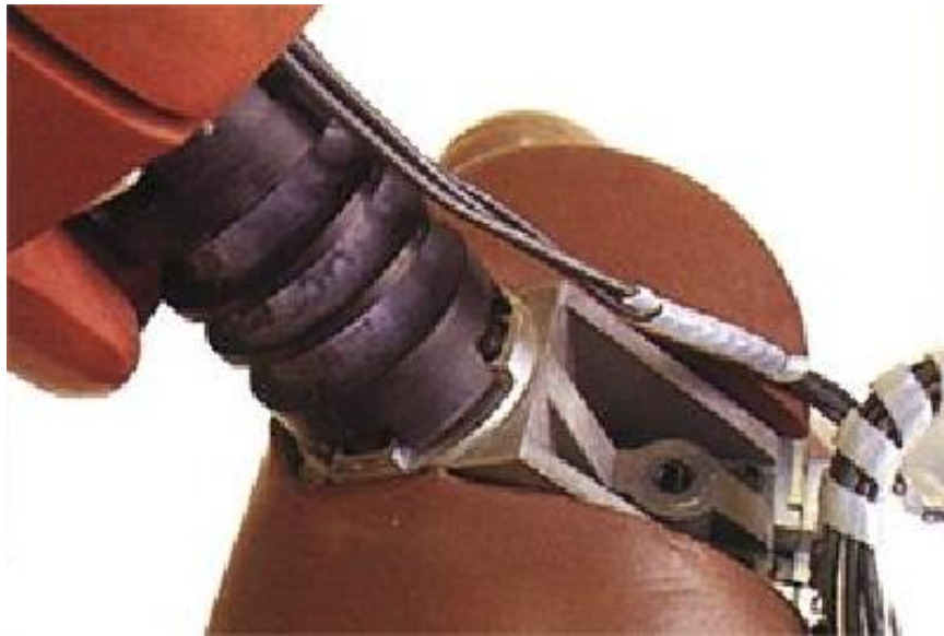
Figure A2. Hybrid III neck sensors (Euroncap 1997)
