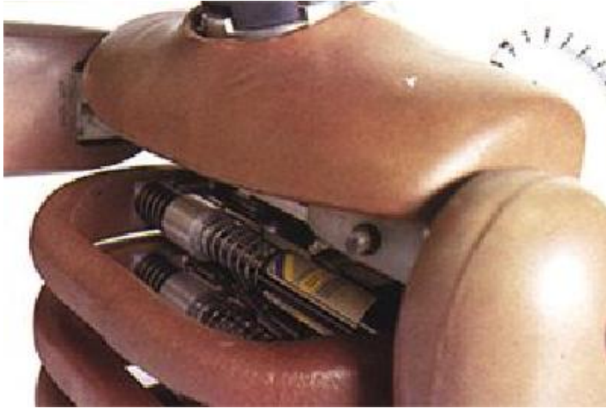
Figure A3. Steel ribs with measuring equipment in upper torso (Euroncap 1997)
