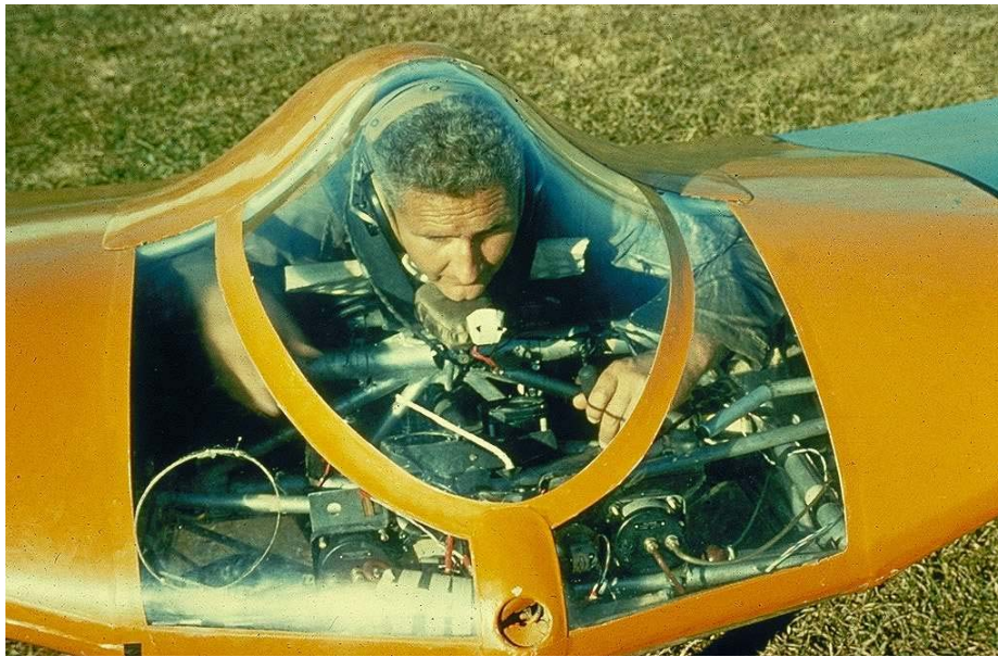
Figure 2.19: A close-up of the Ho IV showing the prone pilot position (RFRL)
