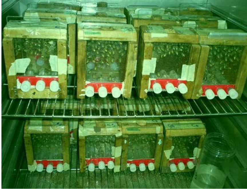
Figure 1: Standard hoarding cages with feeding tubes (plastic tubes with standard windows 2 x 1 cm cut into them), through which bees can access food and water.
