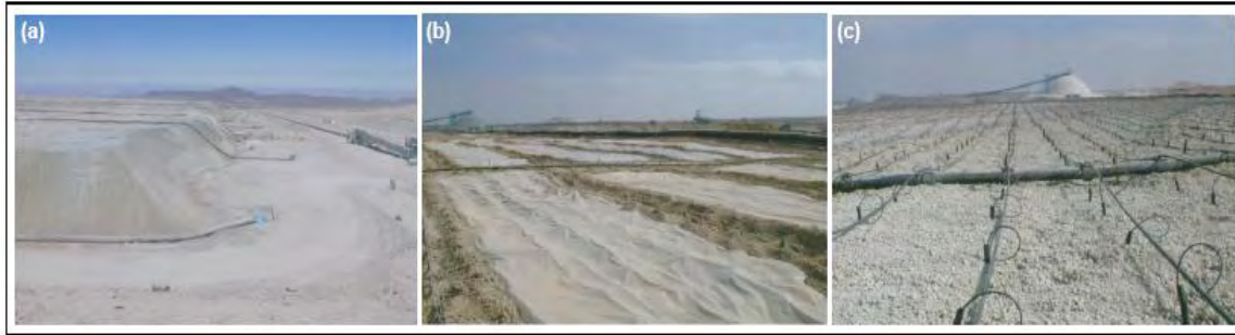
Figure 10. Heap-leaching operation at Cerro Colorado in Chile. (a) Heaps with aeration blowers, (b) insulating thermofilm and (c) buried irrigation drippers (Rawlings et al. , 2003).
