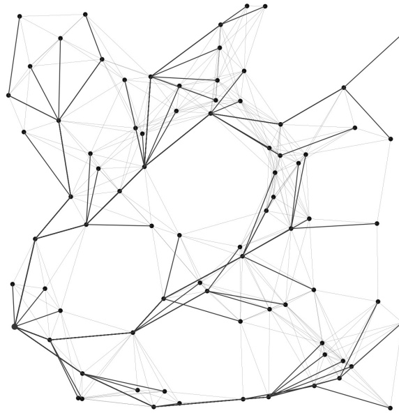
Figure 2.3: Flow load distribution in a 100-node wireless mesh network with equal flow meshing, clearly indicating the central tendency of higher loaded pathways, ideal for network coding without opportunistic listening.
