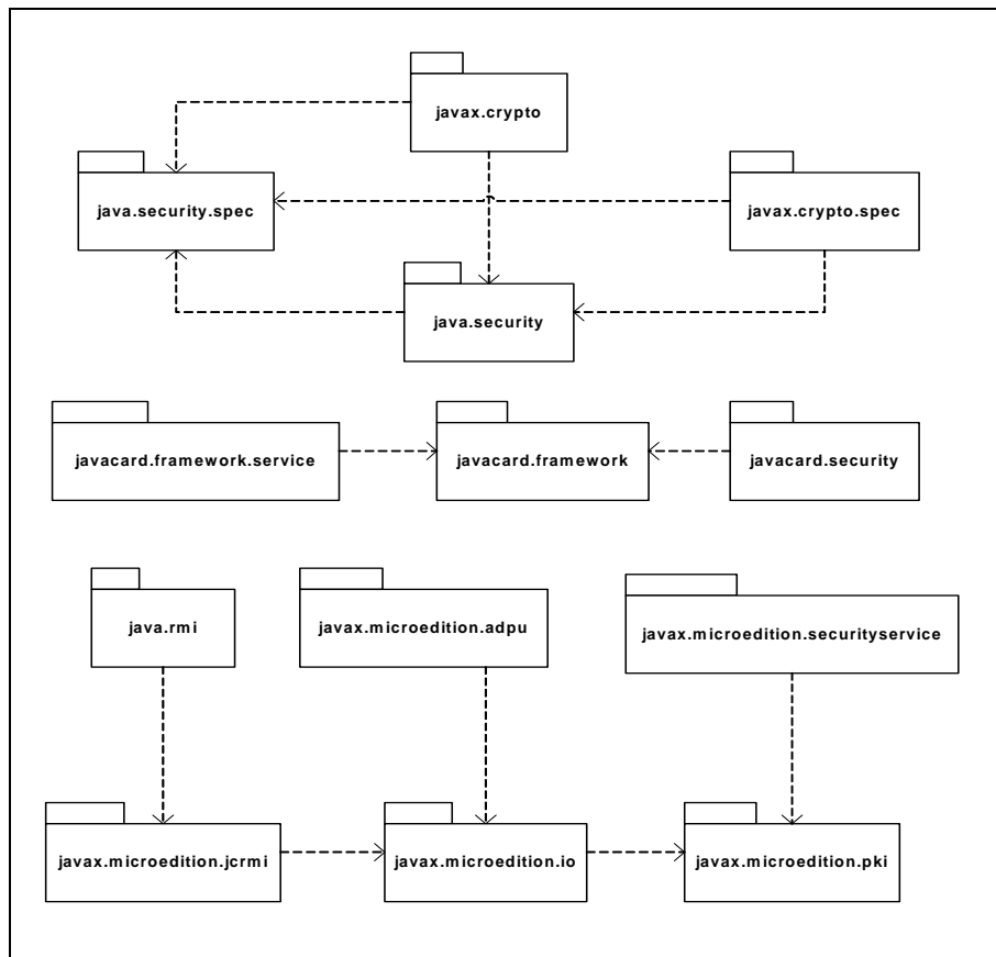
Figure 3-2: Secure and Trust Service API package dependency structure based from SATSA RI 1.0
