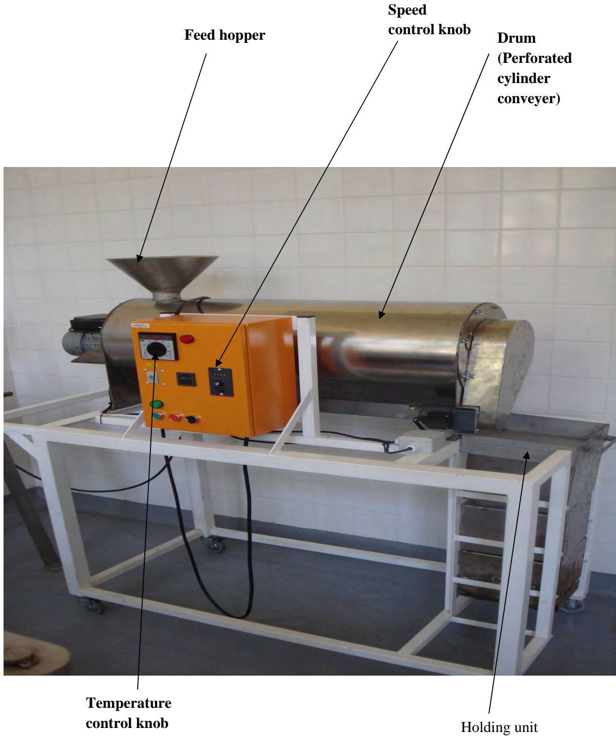
Figure 2.6: Picture of the forced convection continuous tumble roaster used for drying whole marama beans (Roastech, South Africa)
