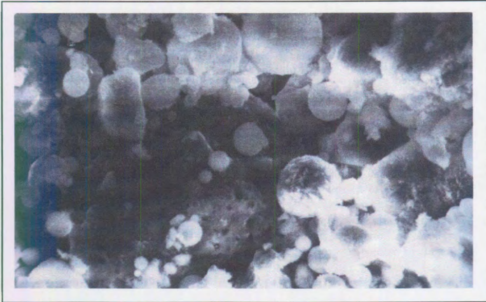
Figure 2.52: SEM micrographic structure of cement paste containing low-calcium fly ash after 4-hours hydration time (Grzeszczyk and Lipowski, 1997).
