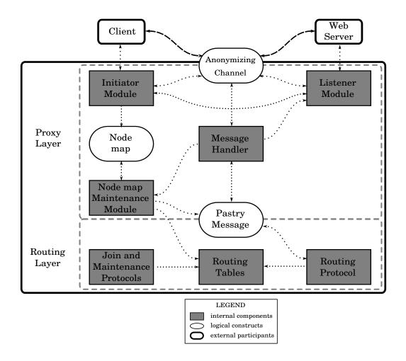
Figure 7.1: Components of a Polar node
