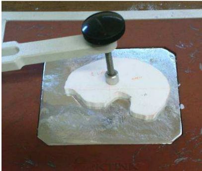
Fig 14 - Cerrobend block mould for electron shielding
