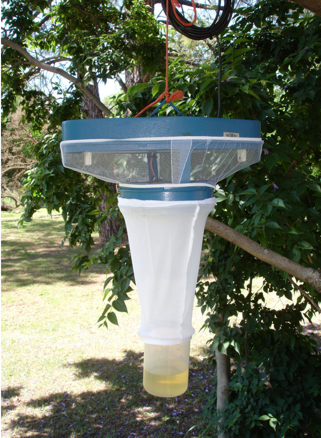
Figure 2.1: A 220 V ultraviolet suction light trap equipped with an 8 W black light tube
