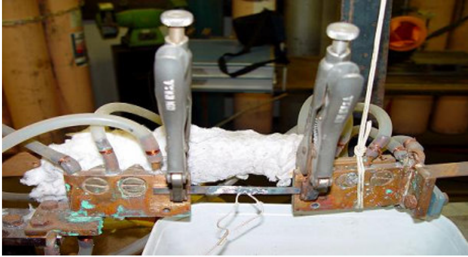
Figure 4.3 - Mounting of the specimen, note that the right hand jaw is suspended to allow free expansion and contraction of the specimen
