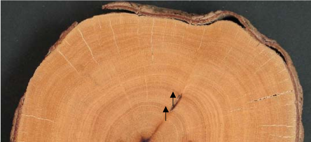
Fig. 3.3. A digital image of a section (pith to bark) of a polished 8 year-old C. equisetifolia stem disk. The black arrows point to two of many dark lines that could denote latewood. All such lines may denote the end of consecutive growth seasons.
