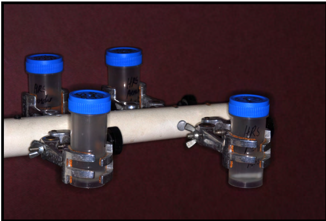
Figure 2.23: Vibromatic (Selecta) was used for constant agitation of the specimens during the demineralizing process.
