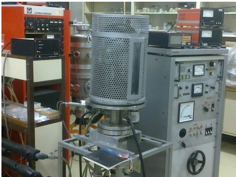
Fig. 3 A picture of the resistive evaporation system.
