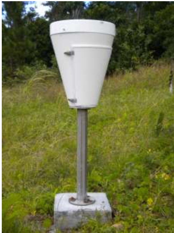
Figure 4.7: Example of the automatic rainfall bucket used by the Mauritius Meteorological Service to record rainfall data.
