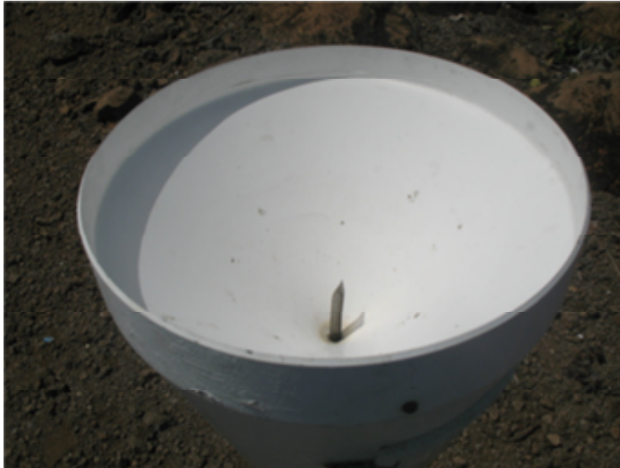
Figure 4.8: Collecting bowl of the rainfall bucket.
