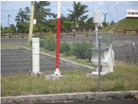
Figure 4.6: Station at Grand Bassin (605m a.s.l.). This particular bucket had an outer covering around the pole but the system is the same.
