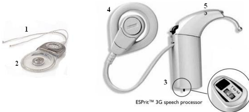
Figure 1.2 ESPrIt 3G and Nucleus 22 cochlear implant system. The components are: 1. The electrode array (which is placed in the inner ear). 2. The receiver for the electrode array. 3. The speech processor 4. Transmitting module and 5. Microphone (worn behind the ear). (Used with permission from http://www.cochlear.com )
