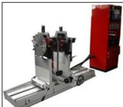
Figure 9: Horizontal Balancing Machine
