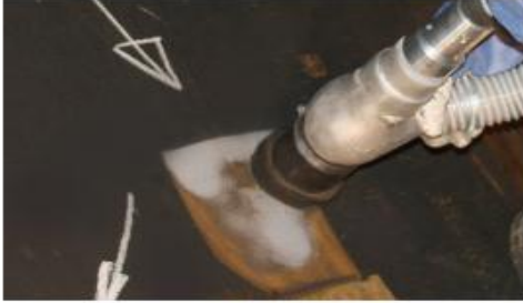
Cleans structures and removes harmful isocyanates that are released during welding and heating
