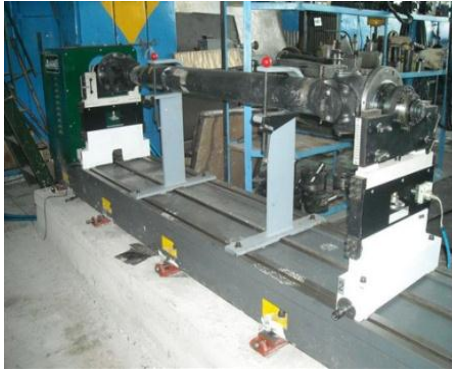
Figure 10: Horizontal Balancing Machine
