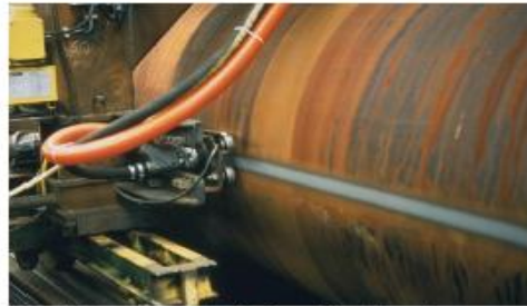
Effectively cleans welding joints without the need of grinding tools
