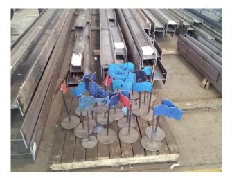
Figure 22: Flags being used to indicate completeness
