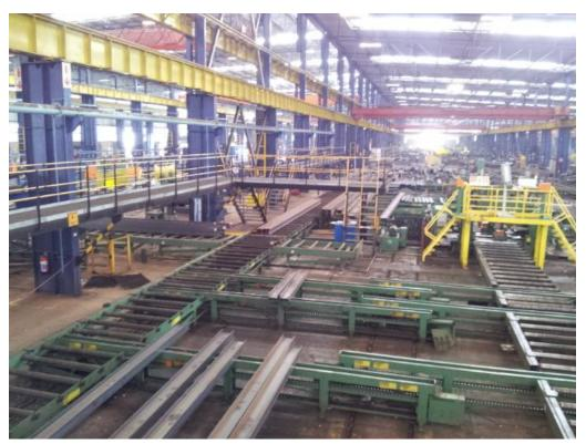
Figure 19: Automated roller conveyor system
