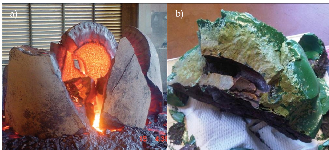
Figure 6: (a) Industrial-scale, high-titania slag block exhibiting distinctly different cooling rates (after Kotze and Pistorius) 11 and (b) slag A after melting and casting, exhibiting distinctly different crystal structures due to different cooling rates similar to the high-titania slag block.
