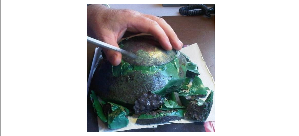
Figure 11: Removing HCFeMn metal that collected at the bottom of the graphite slag pot during cooling of Slag A. The metal was entrapped in the as-received industrial slag during tapping and separated from the slag during re-melting because of the difference in density between the metal and the slag.
