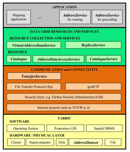
Fig. 2 The Compartimos services in the four main layers of the grid architecture
