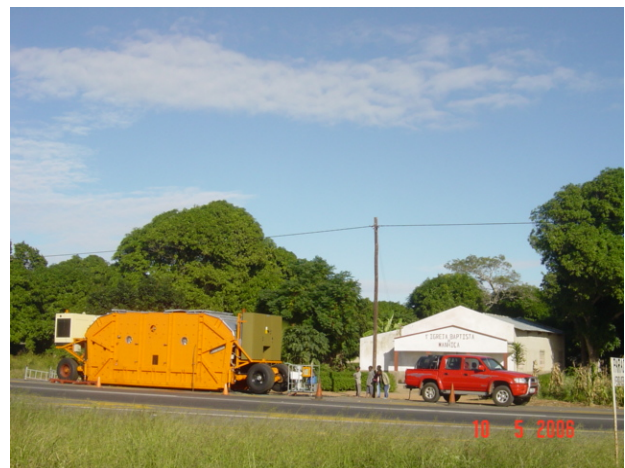
Figure 1: Set-up view of the MLS10 trafficking on the test site at Manhica in Mozambique
