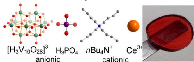
Figure 1: Left: Components required for gel formation: a vanadium oxide source, typically a polyoxovanadate e.g. (n\text{Bu}_4\text{N})_3[\text{H}_3\text{V}_{10}\text{O}_{28}] is dissolved in basic ( (n\text{Bu}_4\text{N})_3\text{OH} -containing) organic solution (e.g. DMSO) and acidified using phosphoric acid in the presence of \text{Ce}^{3+} cations. Instantaneous gelation is observed. Right: photograph of a typical free-standing gel sample.
