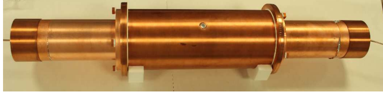
Figure 1. Picture of one of the ANAIS-25 detectors (D0), after the coupling of PMTs and placement of the copper casing at the LSC clean room.
