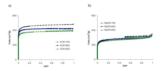
Figure 3. Nitrogen adsorption isotherms of carbons activated with: a) KOH, b) NaOH.
