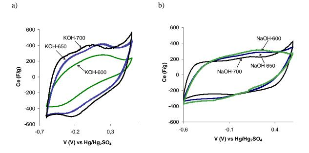
Figure 7. Cyclic voltammograms in a three-electrode cell for: a) KOH and b) NaOH activated carbons.
