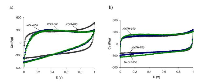
Figure 6. Cyclic voltammograms in a two-electrode cell for: a) KOH and b) NaOH activated carbons.
