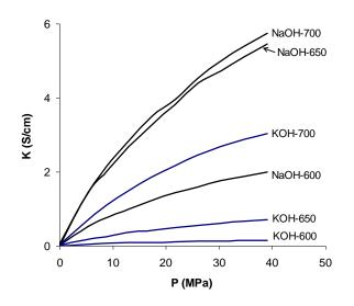
Figure 4. Electrical conductivity values at different pressures.
