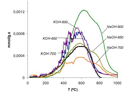
Fig 1. TPD curves corresponding to CO desorption in KOH- and NaOH-activated samples.
