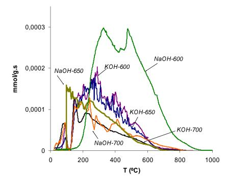
Fig 2. TPD curves corresponding to  $CO_2$  desorption in KOH- and NaOH-activated samples.
