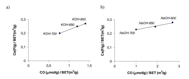
**Figure 8**. Capacitance / BET surface area v.s CO content / BET surface area for: a) KOH-activated samples and b) NaOH-activated samples.
