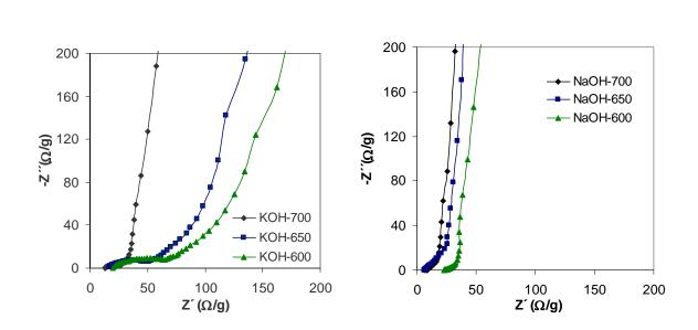
Figure 9. Impedance spectroscopy plot. Extended high frequency region of: a) KOH-activated carbons,b) NaOH-activated carbons.
