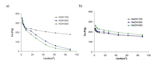
Figure 5. Specific capacitance values vs. current densities for: a) KOH activated carbons, b) NaOH activated carbons.
