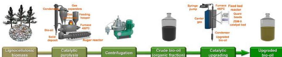
Scheme 1. Overview of the unit operations including all the different steps to produce the aromatic-rich bio-oil from lignocellulosic biomass.
