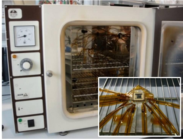
Figure 8. Experimental setup to measure TCR from a packaged device using an oven. Kapton tape is used to avoid short-circuit between contiguous leads of the package. A thermocouple is used to get the temperature measurements while 4-wire resistance measurements of the heater resistance are taken.
