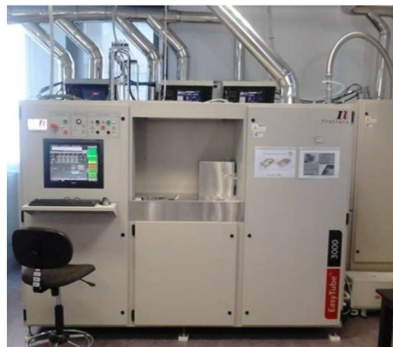
Figure 5: CVD equipment from First Nano, model EasyTube® 3000, located at IREC facilities and used to grow the silicon nanowires by VLS.
