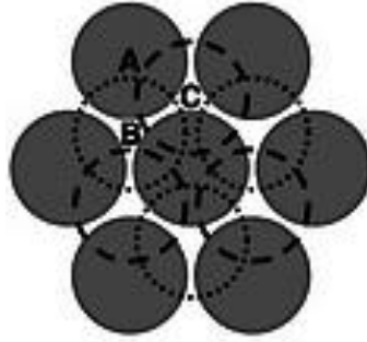
Figure 4.2: Schematic of the ABC stacking sequence for [111] direction of the fcc crystal
