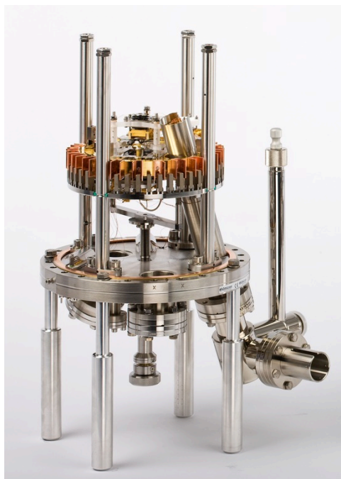
Figure 2.24: Omicron 25K VT STM model used for the experimental STM images taken for this thesis [57].
