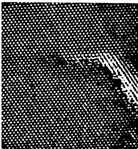
Figure 2.12: An atomically resolved STM image of the Cu(111) surface. Image from Samsavar et al., Phys. Rev. Lett. 65 , 1607-1610, (1990).
