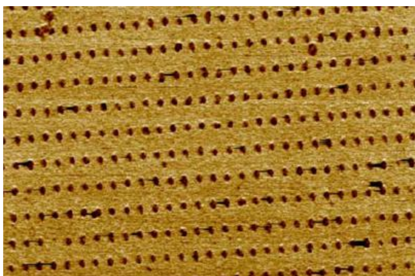
Figure S3 Adhesion-topography coupled images (two different dimensions) of Au nanoparticle (NP) coated with C 8 . The adhesion is strongly suppressed on top of the Au NP.
