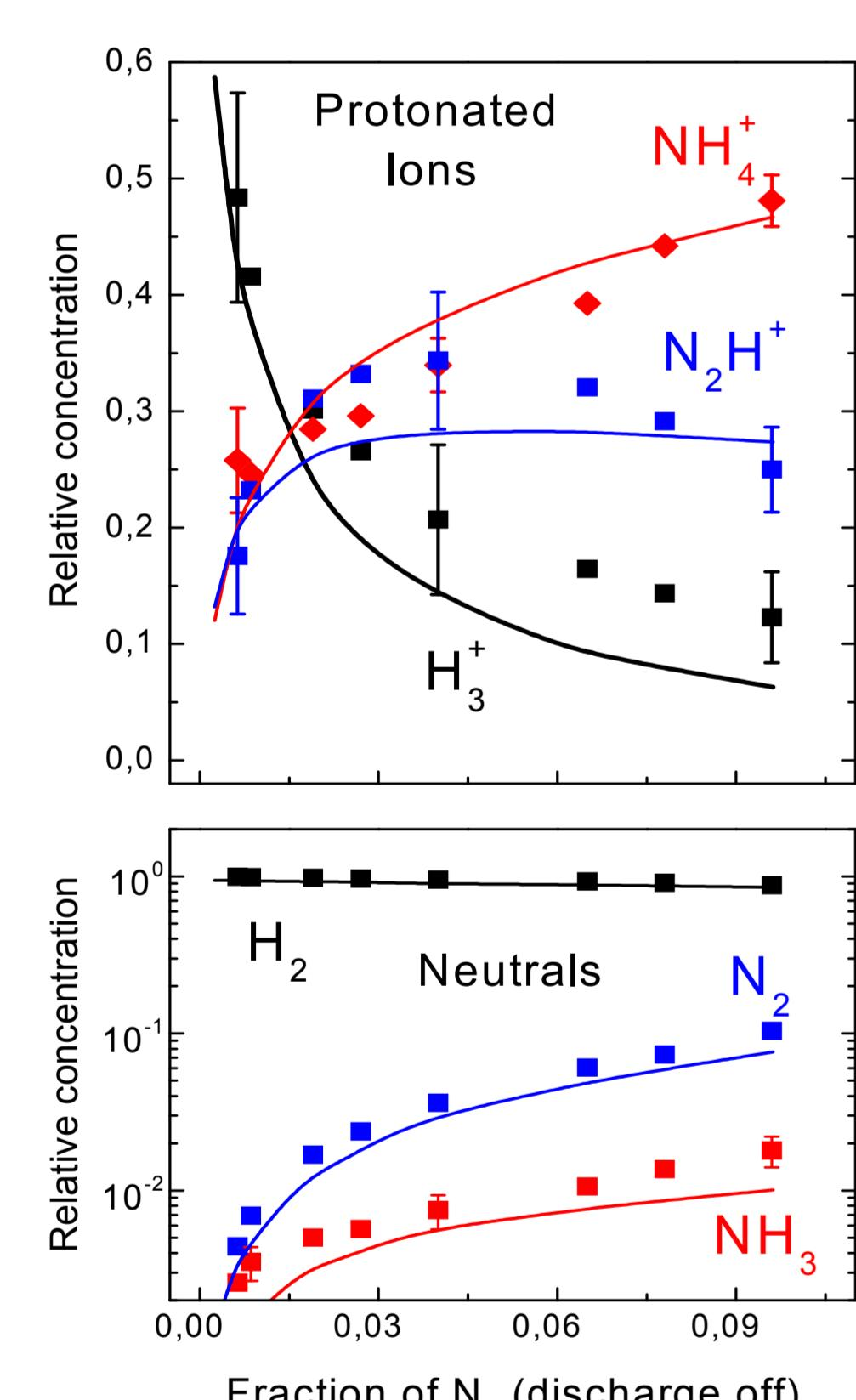
$\text{NH}_4^+$  is derived from the small amount of  $\text{NH}_3$  produced at the reactor walls, and tends to prevail in the ion distributions even for  $\text{NH}_3$  densities  $< 1\%$ .
