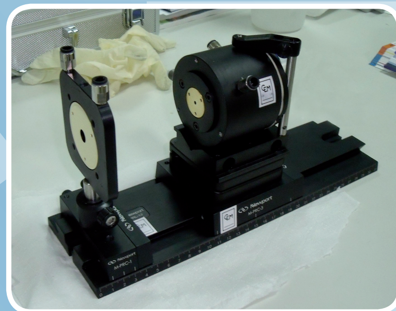
Radiance meter, common for both facilities: trap detector + two precision apertures at a fixed distance
