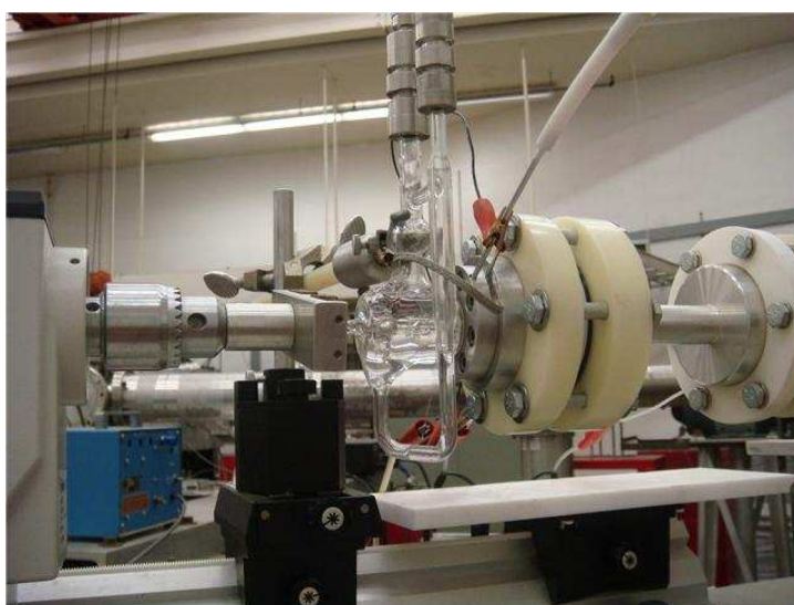
Figure 3.20 Pyrex cell filled with 20 milliliters of the sample (own photo).
