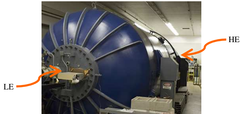
Figure 3.5 Acceleration tank of the FN Van de Graaff accelerator at the Univ. of Notre Dame [6].
