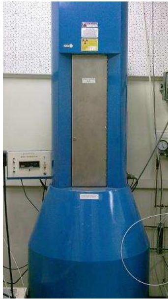
Figure 3.13 The Shepherd 109 cobalt-60 source in the Radiation Laboratory at the University of Notre Dame (own photo).
