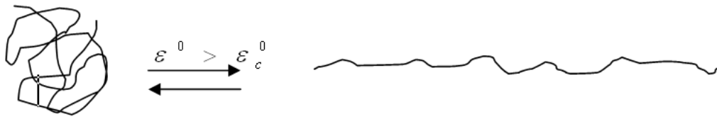
Figure 5.4 Transition from random coil to extended state at a high strain rate 3
