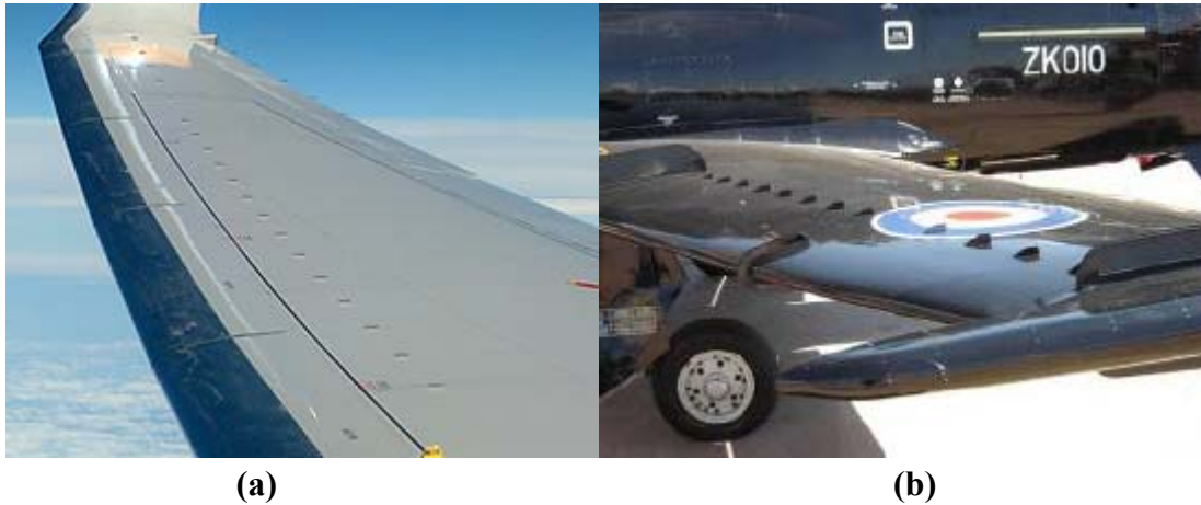
Figure 2.6. The application of Vane Vortex Generators (VVGs) on the wing of (a) an Boeing 757 aircraft ( www.airliners.net ); and (b) a BAE systems Hawk aircraft.
