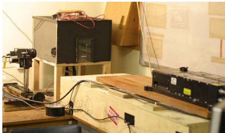
Figure 3.8 The PIV system at quiescent condition
