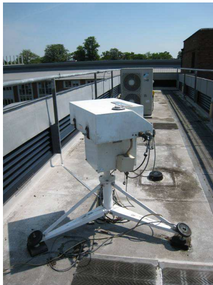
Figure 3.16 The Brewer spectrophotometer (#075) located at the University of Reading.
