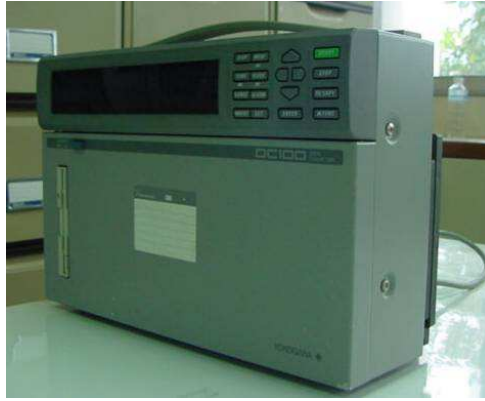
Figure 3.5 A data logger of Yokogawa.
