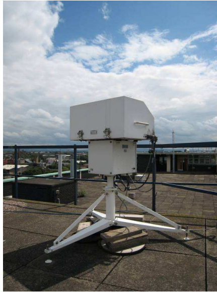
Figure 3.15 The Brewer spectrophotometer (#172) installed at the University of Manchester.
