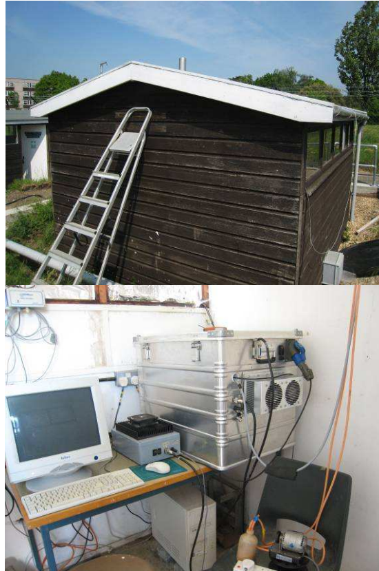
Figure 3.11 The Bentham DMc150 installed at the University of Reading.
