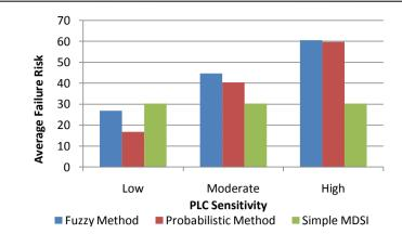
Figure 5-29 Comparison of fuzzy, probabilistic and simple MDSI methods in assessing failure risk of PLC
