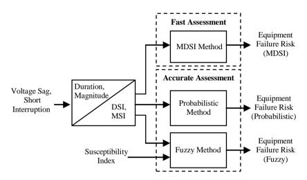
Figure 5-13 Equipment failure risk assessment models
