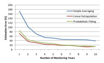
Figure 5-55 Maximum error in voltage sag profile estimation.
