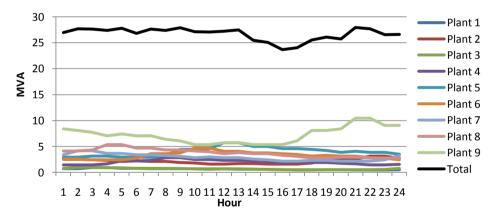
Figure 8-5 Load profile of plants in the HQPZ with optimal loading management
