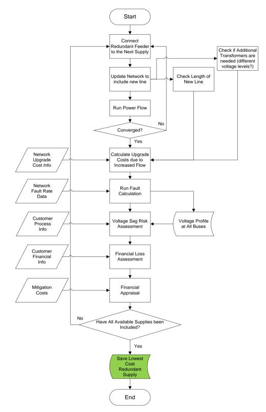
Figure 7-28 Optimal redundant supply assessment flow chart
