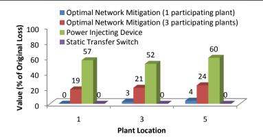
Figure 7-87 The value of optimal network fault reduction with three participating type-37 plants
