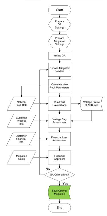
Figure 7-37 Flow chart for optimal reduction of fault frequency and severity
