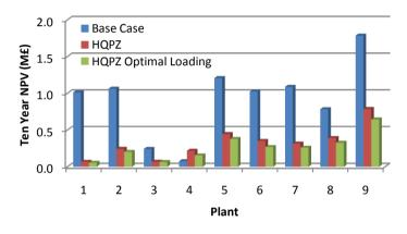
Figure 8-20 Post mitigation losses with redundant supply and power injecting device (30% transmission sags)
