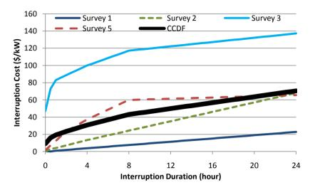
Figure 4-6 Customized customer damage function
