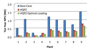
Figure 8-24 Post mitigation losses with best mitigation scheme (10% transmission sags)
