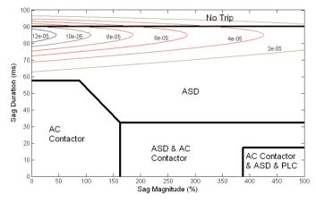
Figure 6-15 Determining of the most vulnerable equipment
