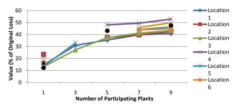
Figure 7-86 The value of optimal network fault reduction for type-16 plants at different plant locations
