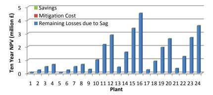
Figure 7-29 Ten year NPV for microprocessor-based processes with redundant supply
