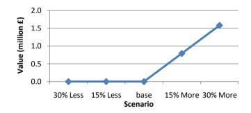
Figure 7-54 Sensitivity of the value shield wires to network fault rates
