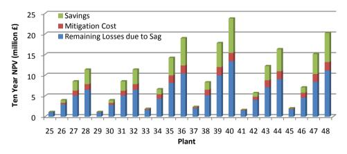
Figure 7-66 Ten year NPV for drive-based processes with optimal network fault reduction
