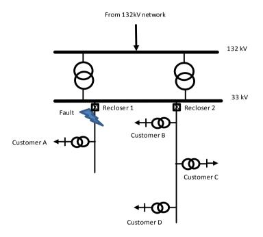
Figure 1-2 Fault caused sags and interruptions
