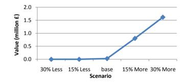
Figure 7-48 Sensitivity of the value of surge arresters to network fault rates
