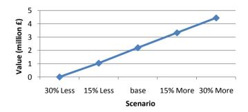
Figure 7-40 Sensitivity of the value of insulating lines to network fault rates
