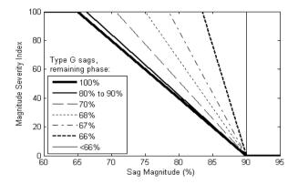
Figure 5-9 Sag magnitude to MSI conversion graph of ASD for type G sags
