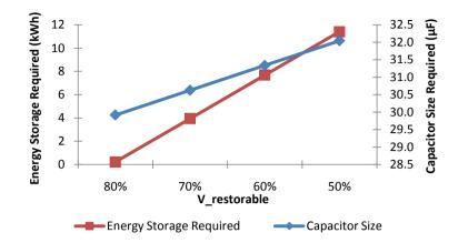
Figure 6-20 Energy storage and capacitor size required for DVR with different restoration capability
