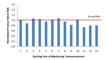
Figure 5-52 Performance estimation with probabilistic fitting method, 5 year monitoring
