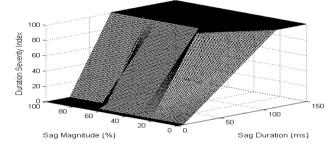
Figure 5-12 DSI conversion graph of AC contactor
