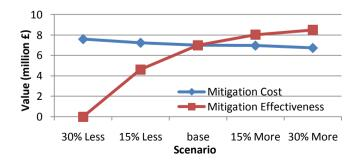
Figure 7-62 Sensitivity of the value of fault current limiting to mitigation cost and effectiveness
