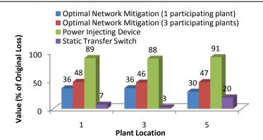
Figure 7-92 The value of optimal network fault reduction with three participating type-40 plants
