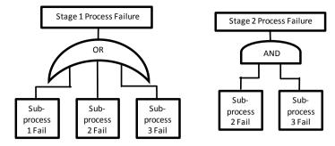
Figure 5-62 Process cycle stage 1 and stage 2 fault trees
