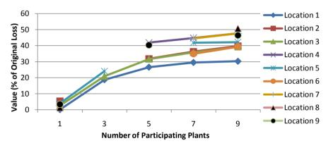
Figure 7-91 The value of optimal network fault reduction for type-37 plants at different plant locations
