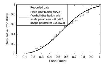
Figure 5-58 Cumulative probability function of office hour type plant
