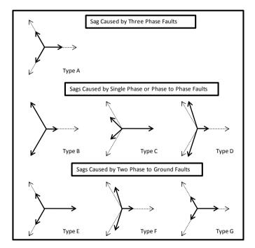
Figure 1-3 Types of voltage sags [6]
