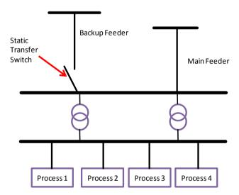
Figure 6-6 Static transfer switch at customer plant
