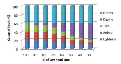
Figure 7-2 Causes of faults for 33kV line
