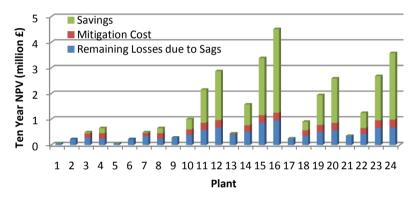
Figure 7-16 Ten year NPV for microprocessor-based processes with installation of power injecting device
