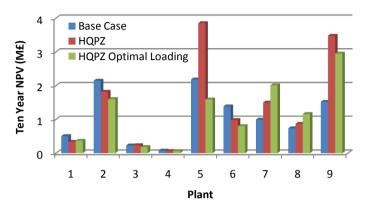
Figure 8-12 Post mitigation losses after installation of power injecting device (30% transmission sags)
