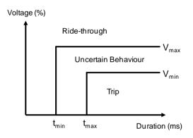
Figure 1-6 General voltage tolerance curve
