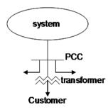
Figure 5-34 customer connection to the grid
