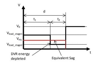
Figure 6-2 Two stage sag and its equivalent
