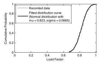
Figure 5-57 Cumulative probability function of continuously operating plant
