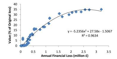
Figure 7-76 Correlation between initial plant loss and the value of optimal fault reduction
