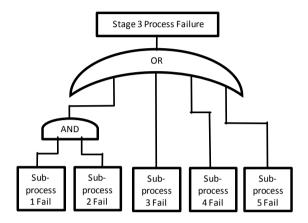
Figure 5-63 Process cycle stage 3 fault tree
