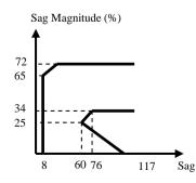
Figure 5-10 Boundaries of AC contactor voltage tolerance. Adopted from [33]
