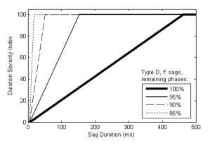
Figure 5-7 Sag duration to DSI conversion graph of ASD for type D, F sags
