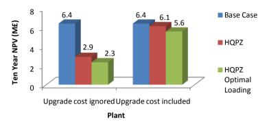
Figure 8-23 Total post mitigation losses with best mitigation scheme (10% transmission sags)
