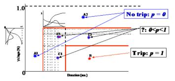
Figure 1-9 Expected behaviour of sensitive equipment against voltage sags of different characteristics. Adopted from [17]
