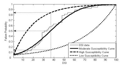
Figure 5-16 Probabilistic model representing duration failure probability
