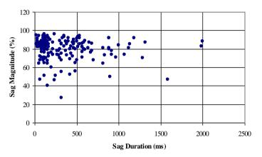
Figure 5-40 Actual 13-year voltage sag profile of a manufacturing plant
