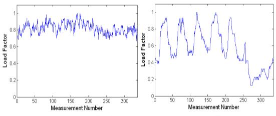
Figure 5-56 Normalized load profile of (a) continuously operating plant (b) office hour type plant
