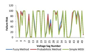
Figure 5-31 Failure risk of ACC with moderate sensitivity for 50 random voltage sag events
