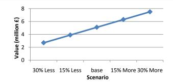
Figure 7-35 Sensitivity of the value of redundant supply to network fault rates
