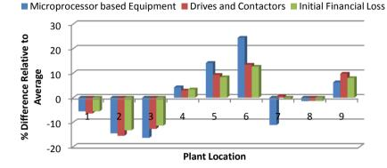
Figure 7-20 Influence of plant location on the value of power injecting device
