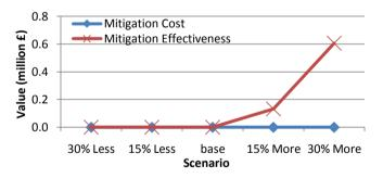
Figure 7-59 Sensitivity of the value of reducing fault clearing time to mitigation cost and effectiveness
