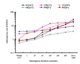
Fig. A-7 Customer damage functions for different high-tech industry categories
