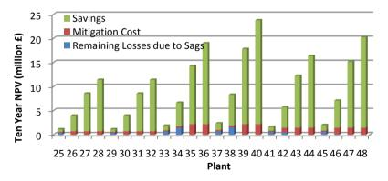
Figure 7-17 Ten year NPV for drive-based processes with installation of power injecting device
