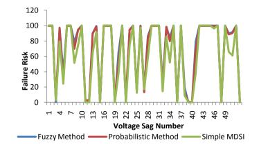
Figure 5-23 Failure risk of ASD with moderate sensitivity for 50 random voltage sag events
