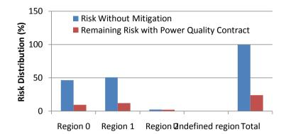
Figure 6-21 The effect of power quality contract on process failure risk
