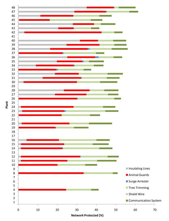
Figure 7-68 Solution mix for plants at Location 6 with optimal network fault reduction
