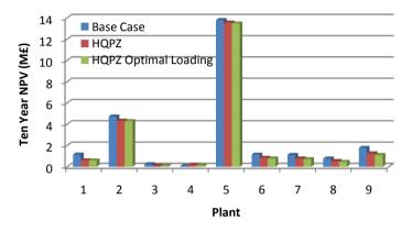
Figure 8-16 Post mitigation losses with redundant supply (30% transmission sags)
