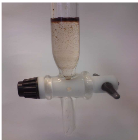
Figure 2. Heavy liquid density separation with heavy particles in the bottom and soil matrix floating on top.
