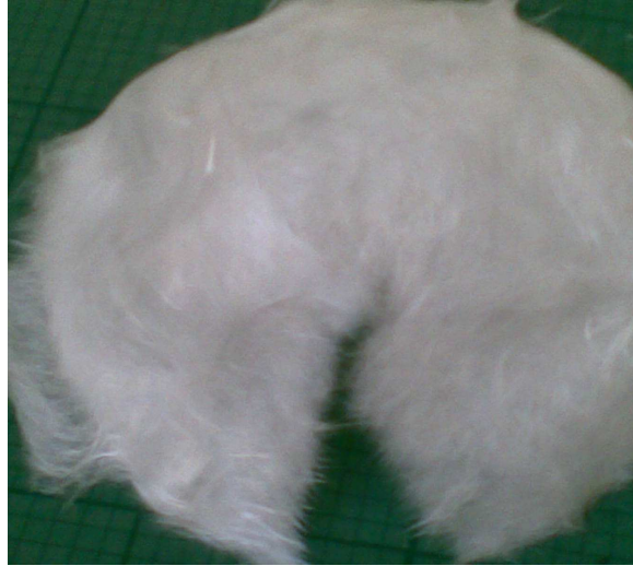
Figure 8.9 3D fibreglass web with a torn side
