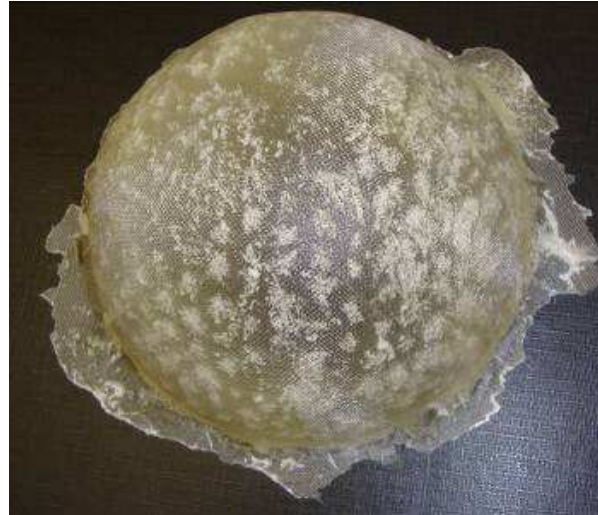
Figure 8.12 Dome shaped 3D fibreglass nonwoven composite sample
