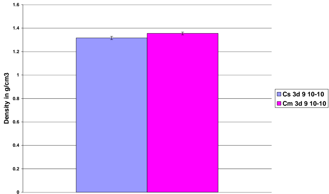
Figure 8.16 Density of different types of 3D composite samples
