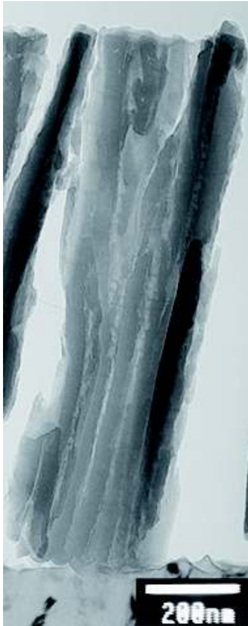
(a) – Anodizing in 0.3 M sulphuric acid solution for 5 min
