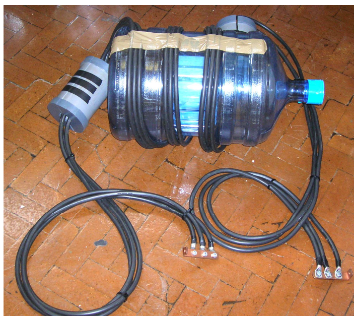
Figure E.5 Photograph of 4.17 \mu H Air core inductor with copper busbars on its terminals used for high current testing on low voltage side of the DAB converter.
