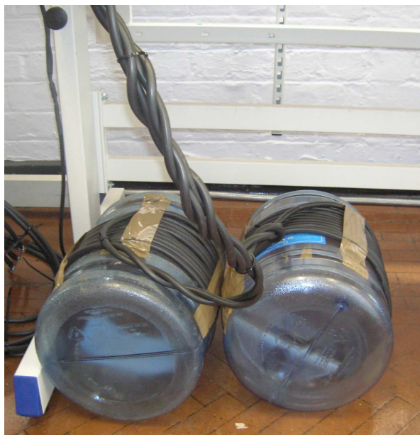
Figure E.4 Photograph of 61.2 \mu H Air core inductor used in DAB converter
