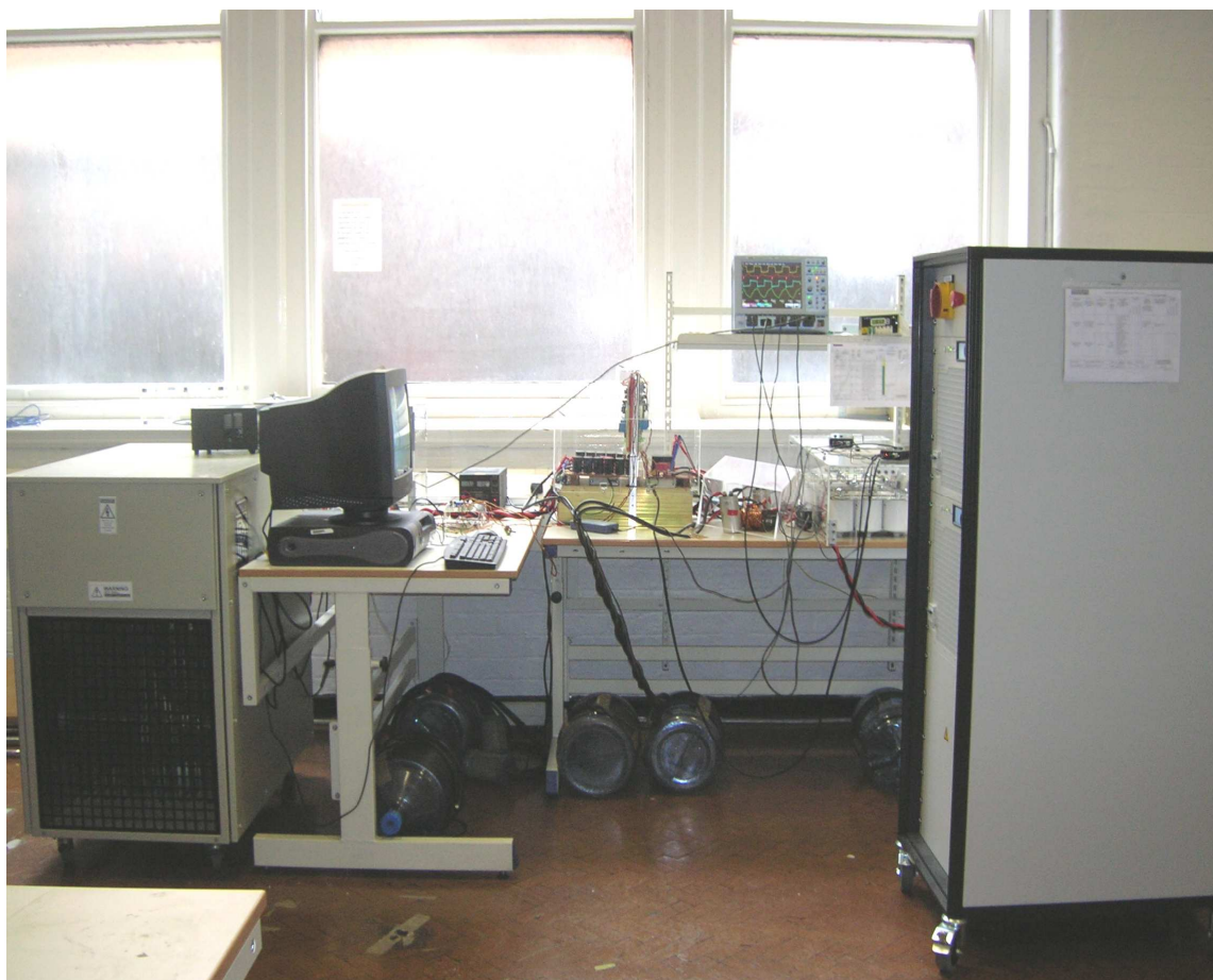
Figure E.1 Photograph of the DAB converter prototype with load bank and high power supply
