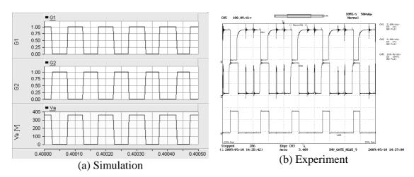
$\label{eq:constraint} \begin{array}{l} Y \mbox{ axis :} Top-G_1 \mbox{ (2V/div-Experiment), Middle}-G_2 \mbox{ (2V/div-Experiment), Bottom}-V_A \mbox{ (100V/div-Simulation, 200V/div-Experiment); X \mbox{ axis: Time (50 $\mu$s/div)} \\ Figure \mbox{ C-20: } G_1 \mbox{ and } G_2 \mbox{ and voltage at node-A} \end{array}$
