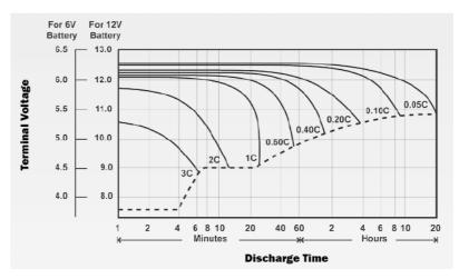
Figure A-3: Discharge characteristics
