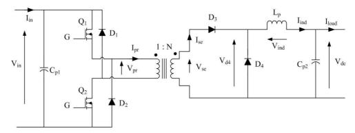
Figure 6-1: Schematic diagram of the modified forward dc-dc converter
