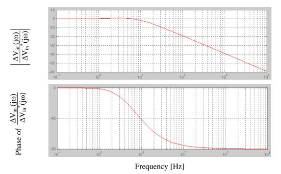
Figure D-7: Command tracking response of the controller
