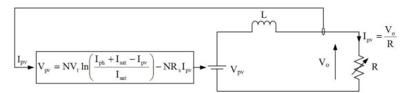
Figure 5-9: Simplified model with the inductor in series with the voltage source
