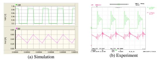
Y axis : $V_{D4}$  - Green (200V/div-simulation, 400V/div-Experiment),  $I_{ind}$  - Pink (0.2A/div) ; X axis: Time (10µs/div) Figure C-4: Voltage across the diode D<sub>4</sub> and the current flowing through the inductor of the modified forward dc-dc converter
