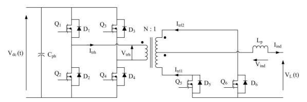
Figure 4-7: Schematic diagram of the bi-directional dc-dc converter
