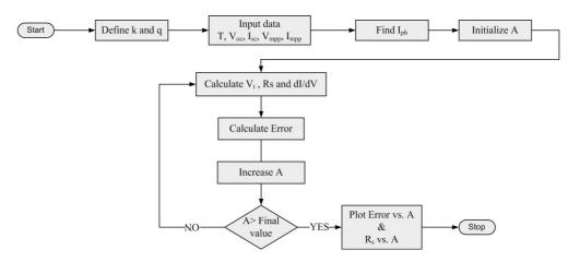
Figure 5-2: Flow chart used to calculate the ideality factor
