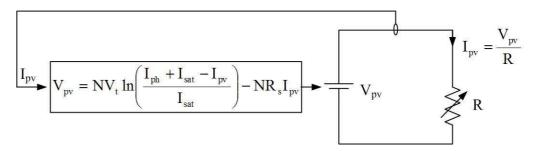
Figure 5-7: Simplified simulation model at constant irradiance and temperature
