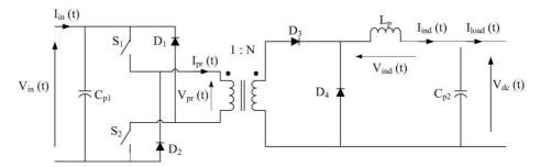
Figure 4-2: Schematic diagram of the modified forward dc-dc converter
