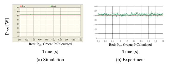
Figure 8-32: Reference and calculated active power variation of inverter
