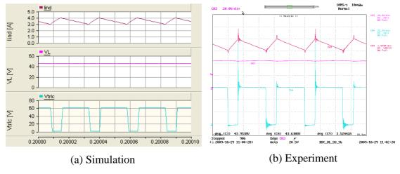
Y axis :  $I_L$  – Brown (1A/div),  $V_L$  – Pink (20V/div),  $V_{trlc}$  – Blue (20V/div) ; X axis: Time (10µs/div) Experimental results:  $I_L$  ground level is same as  $V_L$  ground level
