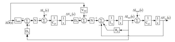
Figure D-3: Operating point state feedback block diagram of the modified forward dcdc converter
