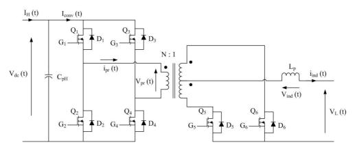
Figure 6-8: Schematic diagram of the bi-directional dc-dc converter
