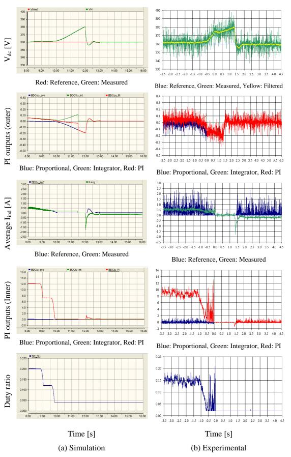
Figure 7-27: Behaviour of the step-up mode controller of the bi-directional dc-dc converter (Automatic step-up mode turn-off transient)
