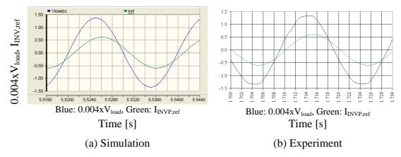
Figure 8-19: Scaled load voltage and inverter current reference
