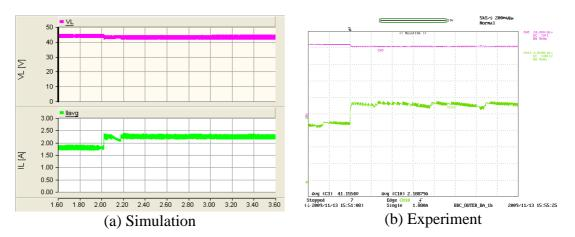
Y axis:  $V_L$  – Pink (10V/div),  $I_L$  – Light green (0.5A/div), Oscilloscope channels bandwidth = 5kHz; X axis: Time (200ms/div)
