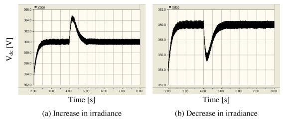
Figure 9-4: Variation of dc-link voltage
