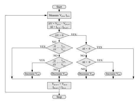
Figure 3-7: Algorithm used in MPPTs based on Incremental conductance method
