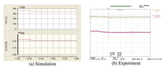
Y axis: V<sub>dc</sub> – Orange (100V/div), I<sub>load</sub> – Maroon (100mA/div – Simulation, 50mA/div-Experimental) Experimental oscilloscope channel bandwidth = 5kHz; X axis: Time (200ms/div)
