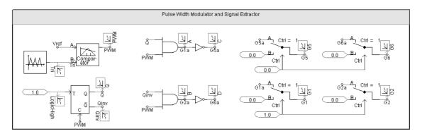
Figure C-13: PWM generator and signal extractor used in the step-down mode of the bidirectional dc-dc converter
