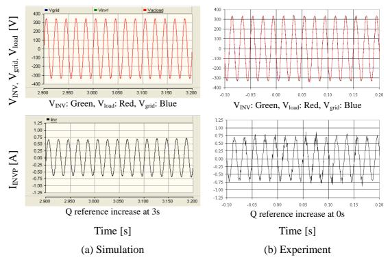
Figure 8-35: Voltages and inverter output current at the increase of reactive power reference
