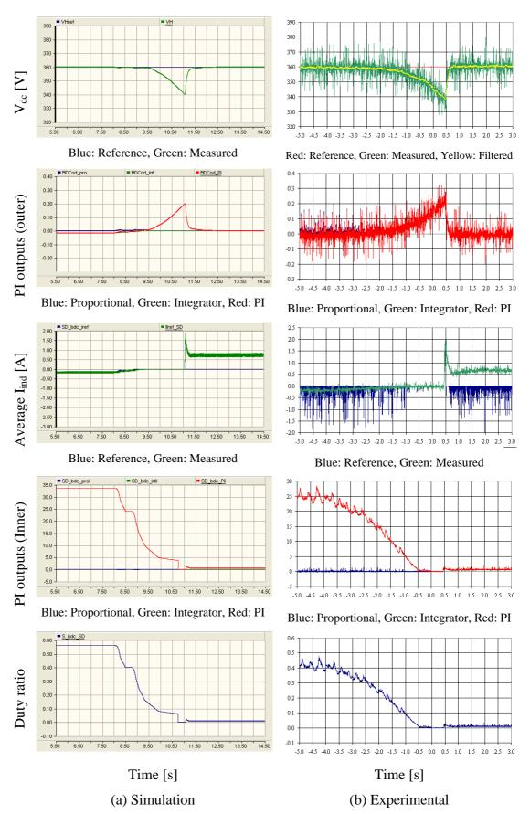
Figure 7-22: Behaviour of the step-down mode controller of the bi-directional dc-dc converter (Automatic step-down mode turn-off transient)
