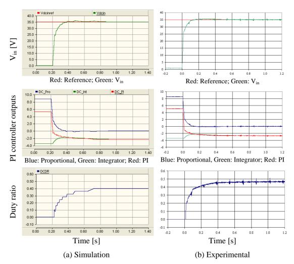
Figure D-11: Response of the controller of the modified forward dc-dc converter
