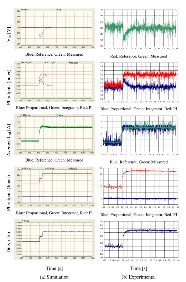
Figure 7-33: Behaviour of the step-up mode controller of the bi-directional dc-dc converter (step-up mode worst-case)
