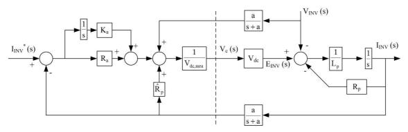
Figure 8-4: Current controller for the single-phase inverter using instantaneous voltage and current measurements
