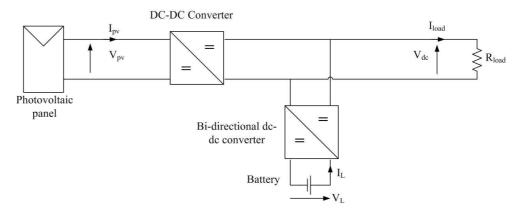
Figure D-26: Integrated test set-up used to test the operation of step-up mode of the bidirectional dc-dc converter
