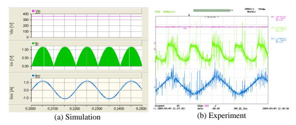
$$\label{eq:Vdiv-Simulation} \begin{split} Y \mbox{ axis } : & V_{dc} - Pink \mbox{ (100V/div-Simulation, 200V/div-Experiment), } I_{in} - Light \mbox{ green (0.5A/div), } I_{INV} - \\ & Blue \mbox{ (1A/div); } X \mbox{ axis: Time (5ms/div)} \end{split}$$
