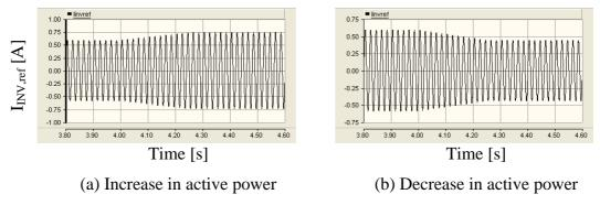
Figure 9-9: Inverter current reference
