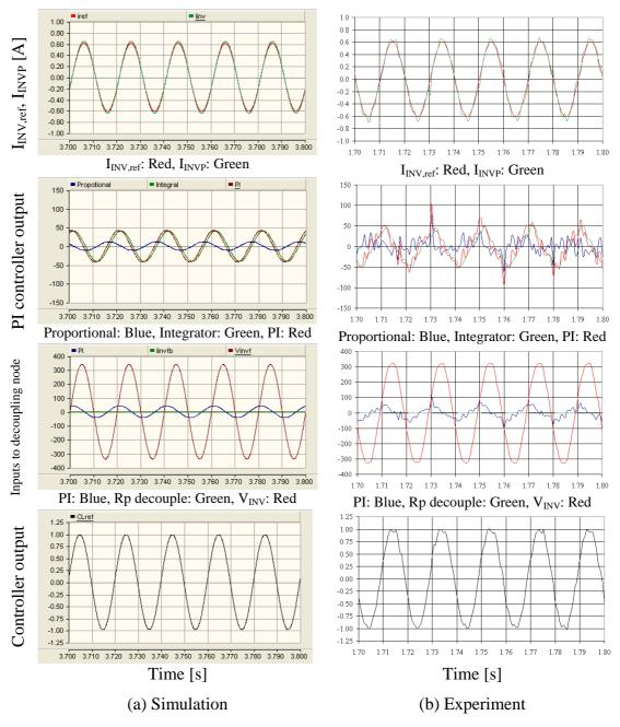
Figure 8-21: Behaviour of the current controller after the grid connection
