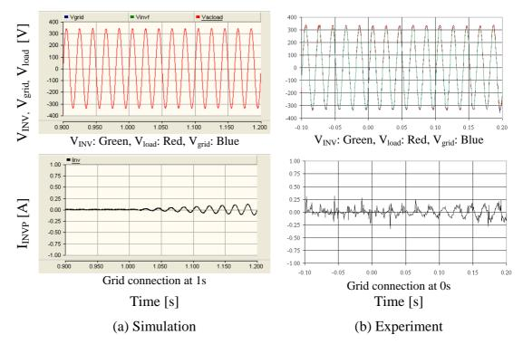
Figure 8-28: Voltages and inverter output current during the grid connection
