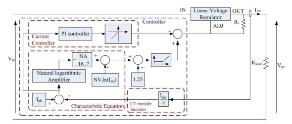
Figure 5-22: Photovoltaic emulator with additional circuitry which behaves properly at low voltages
