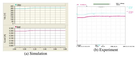
Y axis: V<sub>dc</sub> – Light blue (50V/div), I<sub>load</sub> – Brown (50mA/div) Experimental oscilloscope channel bandwidth = 5kHz; Ground level of CH4 and CH9 are same in experimental results; X axis: Time (100ms/div) Figure D-27: Load current and dc-link voltage during the transient
