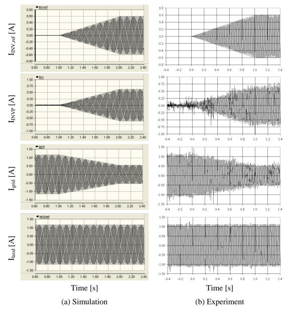
Figure 8-27: Inverter current reference and currents flowing through the inverter, load and grid
