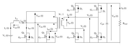
Figure C-5: Test set-up used to the operation of the step-up mode of the bi-directional converter
