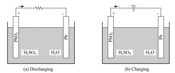
Figure A-2: Structure of a Lead acid battery [A8]
