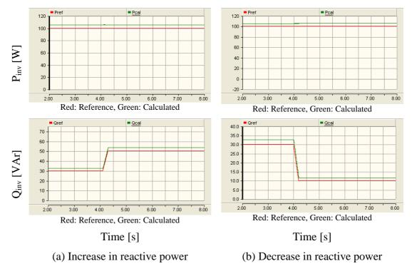
Figure 9-25: Active and reactive power outputs of the inverter
