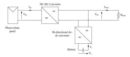
Figure D-39: Test set-up for outer voltage loop of bi-directional dc-dc converter during step-down mode
