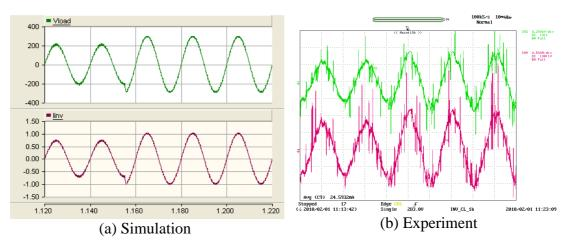
$Y \ axis: \ V_{INV} - Green \ (200V/div), \ I_{INV} - Maroon \ (0.5A/div); \ X \ axis: \ Time \ (200ms/div); \ Step \ change: \ just \ before \ 1.16 \ in \ simulation, \ at \ the \ beginning \ of \ 4^{th} \ time/div \ block \ in \ experimental$
