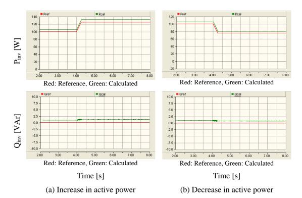
Figure 9-11: Active and reactive power output of the inverter
