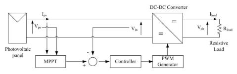
Figure 7-2: Controller of the modified forward dc-dc converter
