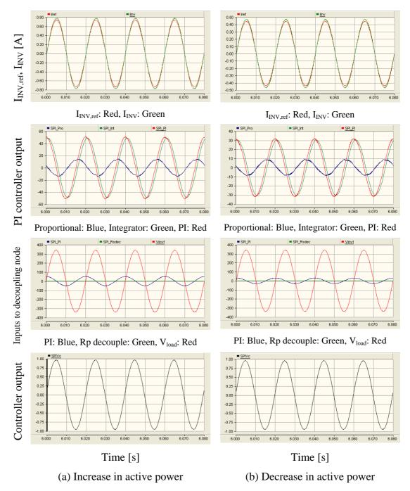
Figure 9-17: Behaviour of the current controller of the inverter
