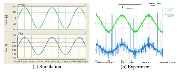
Y axis :V<sub>IINV</sub> – Green (200V/div), I<sub>IINV</sub> – Blue (simulation: 0.5A/div, experiment: 1A/div); X axis: Time (5ms/div) Figure 6-27: Voltage across the load and current flowing through the load
