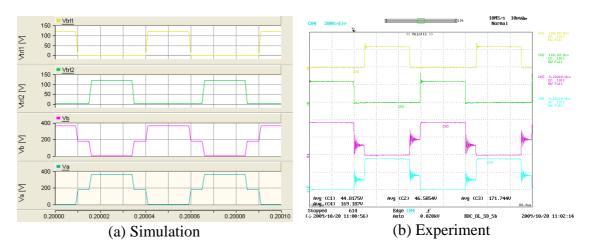
Y axis :V<sub>trl1</sub> – Light yellow (50V/div-simulations, 100V/div-Experiment), V<sub>trl2</sub> – Green (50V/div-simulations, 100V/div-Experiment), V<sub>a</sub> – Pink (200V/div), V<sub>b</sub> – Light blue (200V/div); X axis: Time (10µs/div) Figure C-14: Voltage across the primary and secondary windings of the bi-directional dc-dc converter (step-down mode)
