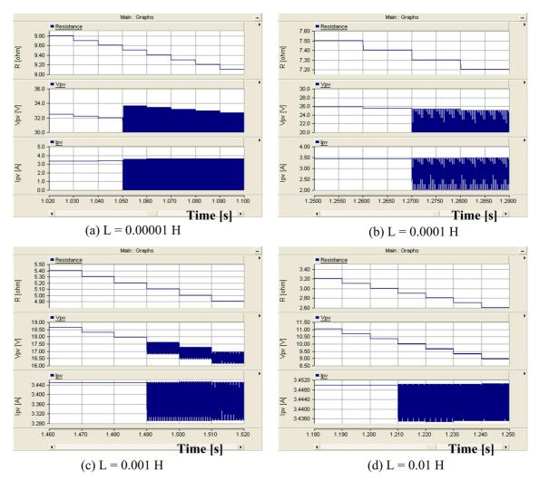
Figure 5-12: Failure point of the simulation model of the photovoltaic panel for different inductance values
