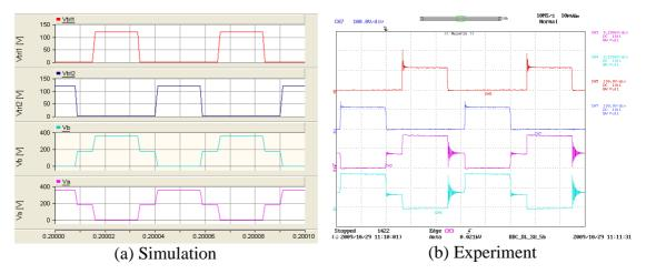
Y axis :V<sub>trl1</sub> – Light brown (50V/div-Simulations, 100V/div-Experiment), V<sub>trl2</sub> – Dark blue (50V/div-Simulations, 100V/div-Experiment), V<sub>a</sub> – Pink (200V/div), V<sub>b</sub> – Light blue (200V/div); X axis: Time (10µs/div) Figure C-10: Voltage across switches Q<sub>2</sub>, Q<sub>4</sub>, Q<sub>5</sub> and Q<sub>6</sub> of the bi-directional converter (step-up mode)
