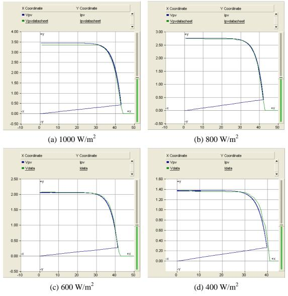
Y-axis: Current [A], X-axis: Voltage [V]; Blue: Simulation model, Green: Datasheet Figure 5-13: Comparison of characteristic curves at 25°C for different irradiance conditions
