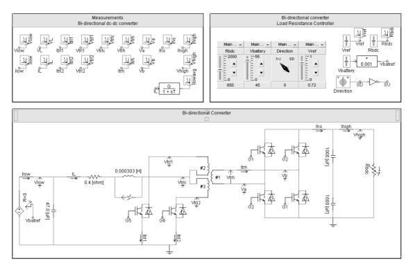
Figure C-6: Screen capture of the simulation model of the bi-directional dc-dc converter in step-up mode
