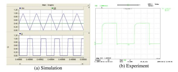
Y axis: Simulations – [top: V<sub>tri</sub> and Duty ratio, Bottom: Gate signal], Experimental – [Gate signal to G<sub>1</sub>: Green (1V/div)]; X axis: Time (Simulations: 20µs/div, Experiment: 5µs/div)
