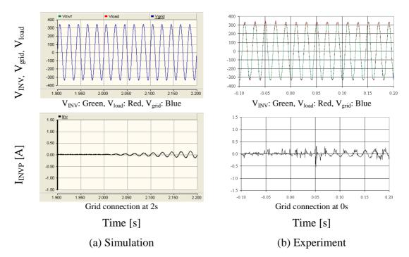
Figure 8-14: Load voltage and inverter output current at the point of grid connection
