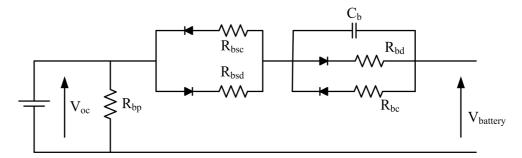
Figure A-9: Modified thevinin's equivalent circuit of a battery
