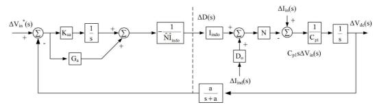
Figure D-4: State feedback block diagram of the controller of the modified forward dcdc converter
