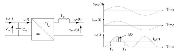
Figure 4-18: Inverter output current and principle input current
