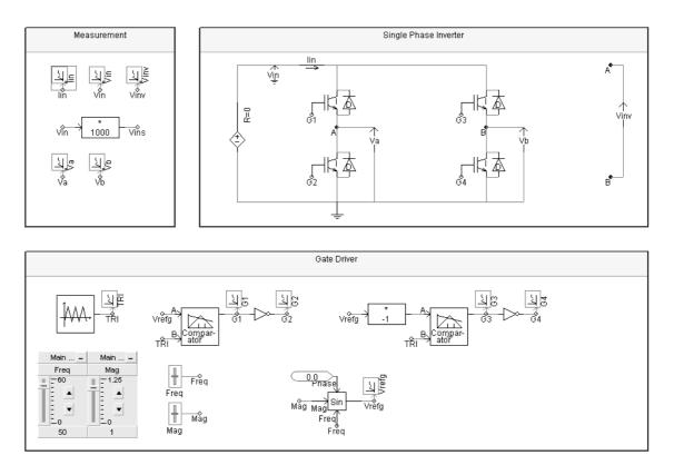
Figure C-19: Screen capture of the single-phase inverter operated in no-load condition
