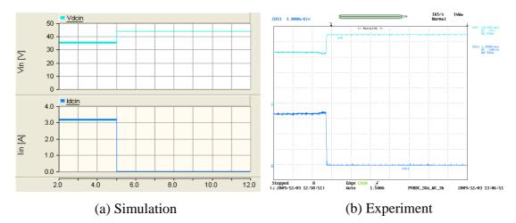
Figure 7-29: Photovoltaic panel voltage and current (Step-up mode worst-case)
