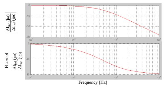
Figure D-16: Command tracking response of the inner current loop
