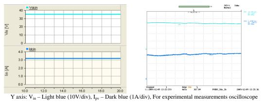
channels bandwidth = 5kHz,; X axis: Time (1s/div)
