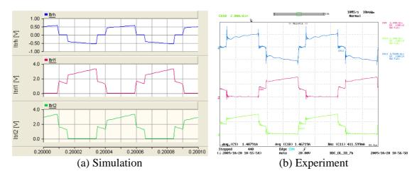
Y axis :I<sub>trh</sub> – Blue (0.5A/div), I<sub>trl1</sub> – Brown (2A/div), I<sub>trl2</sub> – Green (2A/div); X axis: Time (10µs/div) Figure C-15: Currents flowing through the windings of the transformer of the bidirectional dc-dc converter (step-down mode)
