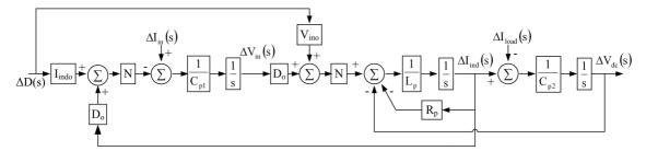
Figure 4-6: State feedback block diagram of the modified forward dc-dc converter based on the operating point state equations
