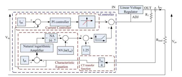
Figure 5-23: Final model of the photovoltaic emulator
