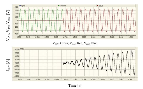
Figure 9-30: Inverter load current and load voltage
