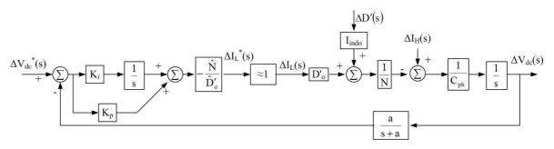
Figure D-19: Outer control loop of the bi-directional dc-dc converter at step-up mode
