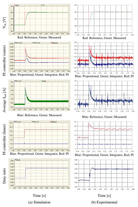
Figure D-29: Behaviour of the bi-directional dc-dc converter controller during the stepup mode
