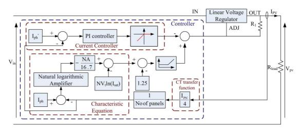
Figure 5-25: Photovoltaic emulator capable of emulating five photovoltaic panels
