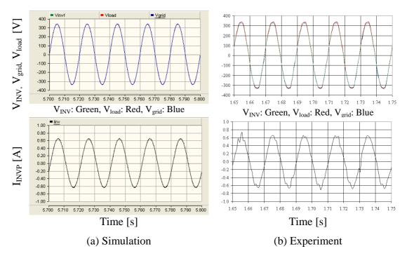
Figure 8-24: Load voltage and inverter output current after grid connection
