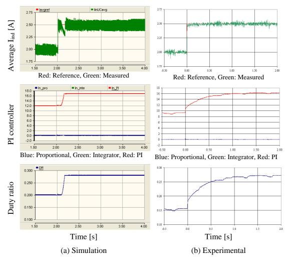
Figure D-17: Behaviour of the inner current controller of the bi-directional dc-dc converter at step-up mode
