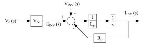
Figure 4-17: State feedback block diagram of the system
