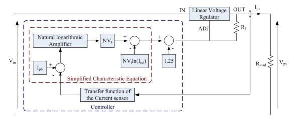
Figure 5-18: Block diagram of the photovoltaic emulator with simplified characteristic equation of the photovoltaic panel
