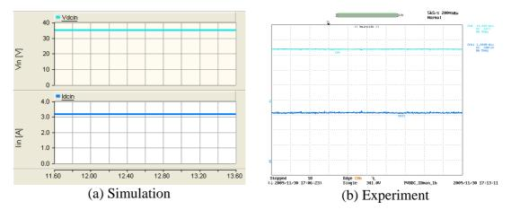
Y axis:  $V_{dcin}$  – Light blue (10V/div),  $I_{pv}$  – Dark blue (1A/div), Experimental results oscilloscope channel bandwidth = 5kHz; X axis: Time (200ms/div)
