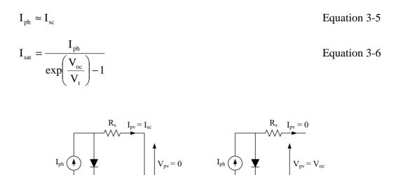
Figure 3-5: Photovoltaic cell under open circuit and short circuit test condition
