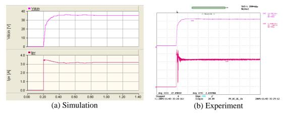
$$\label{eq:Variation} \begin{split} \text{Y axis: } V_{\text{in}} - \text{Pink (10V/div), } I_{\text{pv}} - \text{Maroon (1A/div), Experimental results oscilloscope channel} \\ \text{bandwidth} = 5 \text{kHz; X axis: Time (200ms/div)} \end{split}$$
