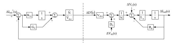
Figure D-13: Inner current loop for the bi-directional dc-dc converter
