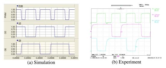
Y axis :Simulations – [Top: PWM, Middle: Q<sub>5</sub>, Bottom: Q<sub>6</sub>], Experiment - [Top: PWM - Green (2V/div), Middle - Q<sub>5</sub> - Pink (5V/div), Bottom - Q<sub>6</sub> - Blue (5V/div)] ; X axis: Time (10µs/div) Figure 6-13: Gate signal applied during step-up mode of bi-directional dc-dc converter
