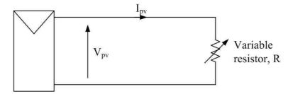
Figure 5-5: Test set-up used to test the simulation of the photovoltaic panel
