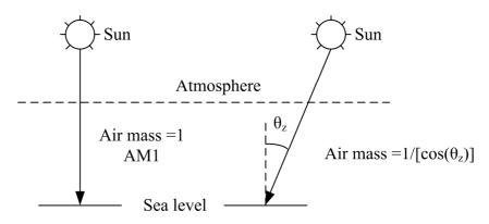
Figure 3-1: Air mass depending on the sunlight path
