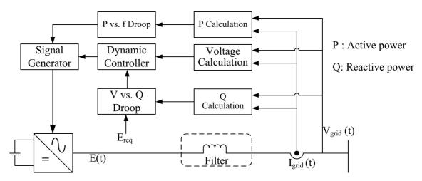
Figure 2-9: Microsource controller used in CERTS MicroGrid without master-slave control
