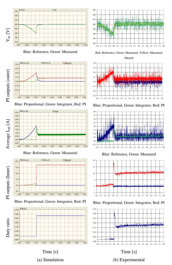
Figure 7-16: Behaviour of the step-up mode controller of the bi-directional dc-dc converter (Automatic step-up mode turn-on transient)
