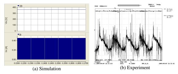
Y axis :Top -  $V_{dc}$  (100V/div), Bottom –  $I_{dc}$  (0.2A/div); X axis: Time (5ms/div) Figure C-28: Input voltage and input current flowing through the inverter
