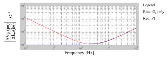
Figure D-15: Dynamic stiffness response of the inner current controller
