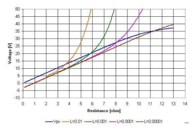
Figure 5-11: Variation of convergence limit with load resistance for different inductor values and output voltage of the photovoltaic panel  $(V_{pv})$  with load resistance
