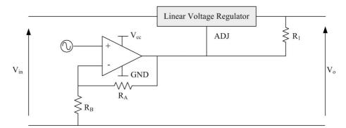
Figure 5-15: Feasibility testing of adjustable voltage regulator for the application of PV Emulator
