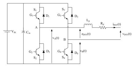
Figure 4-16: Single-phase inverter connected to grid through a coupling inductor showing definition of variables
