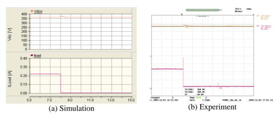
$Y \ axis: \ V_{dc} - Orange \ (50V/div-simulations, \ 100V/div-Experiment), \ I_{load} - Maroon \ (0.1A/div) \ Experimental \ oscilloscope \ channel \ bandwidth = 5kHz,; \ X \ axis: \ Time \ (1s/div)$
