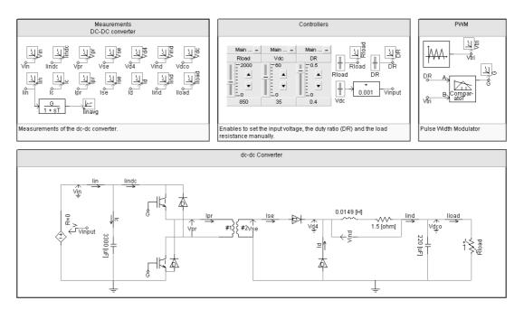
Figure C-2: Screen capture of the simulation model of the modified forward dc-dc converter
