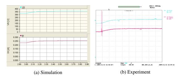
Y axis: V<sub>dc</sub> – Light blue (50V/div), I<sub>load</sub> – Maroon (50mA/div) Experimental oscilloscope channel bandwidth = 5kHz; X axis: Time (100ms/div) Figure D-23: DC-link voltage and load current
