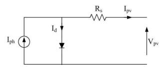
Figure 5-1: Photovoltaic cell model used to develop simulation model
