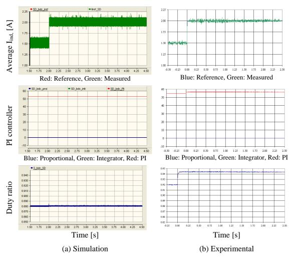
Figure D-35: Behaviour of the inner current control loop of the bi-directional dc-dc converter during step-down mode
