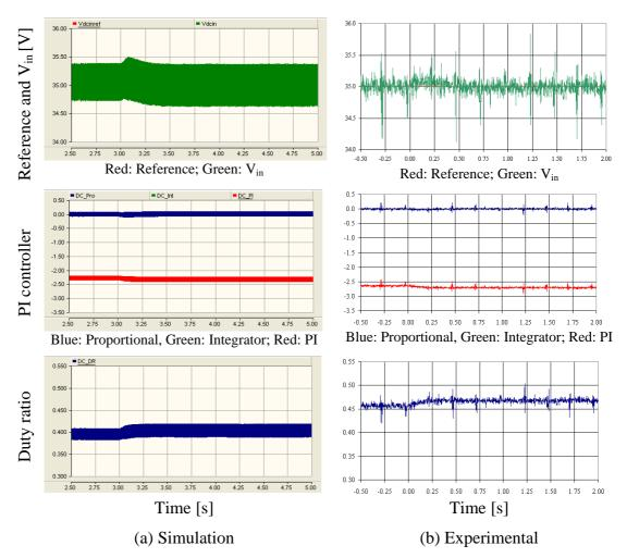
Figure D-31: Behaviour of the controller of the modified forward dc-dc converter
