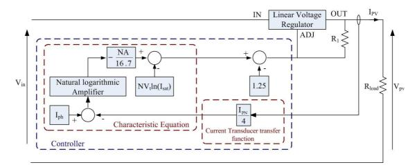
Figure 5-21: Block diagram of the photovoltaic emulator based on Equation 5-33 and current transducer transfer function
