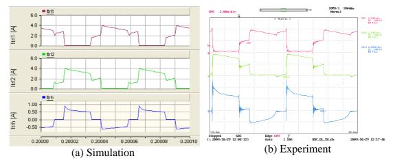
Y axis :  $I_{trl1}$  – Light brown (2A/div),  $I_{trl2}$  – Light green (2A/div),  $I_{trh}$ – Light blue (0.5A/div) ; X axis: Time (10µs/div)
