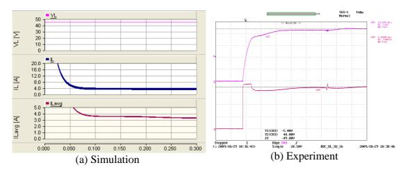
Y axis :V<sub>L</sub> - Pink (10V/div), I<sub>L</sub> – Maroon (1A/div) ; X axis: Time (50ms/div-Simulation,1s/div-Experiment) Figure 6-15: Voltage at the low-voltage end of the converter and input current to the bidirectional dc-dc converter (step-up mode)
