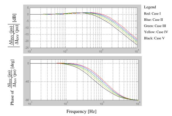
Figure 8-7: Command tracking response of the current controller for the selected cases
