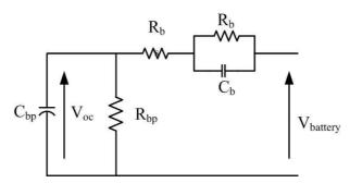
Figure A-10: Lead-acid battery electrical model
