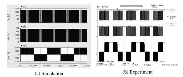
Y axis :Top –  $V_A$  (100V/div-Simulation, 200V/div-Experiment), Middle –  $V_B$  (100V/div, 200V/div-Experiment), Bottom –  $V_{INV}$  (200V/div); X axis: Time (5ms/div)
