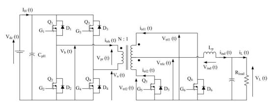
Figure C-11: Test set-up used to test the operation of the step-down mode of the bidirectional dc-dc converter
