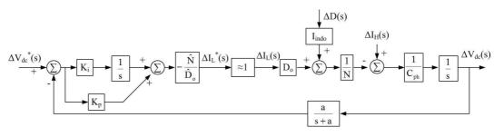
Figure D-37: Outer voltage control loop of the bi-directional dc-dc converter during step-down mode
