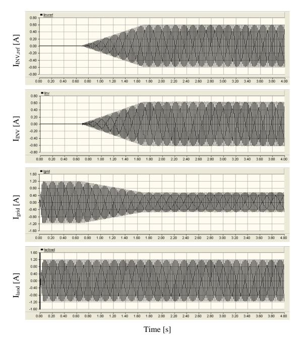
Figure 9-29: Inverter output current reference, inverter output current, grid current and load current
