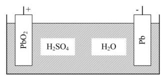
Figure A-1: Structure of a lead-acid battery
