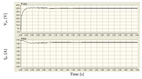
Figure 9-26: Photovoltaic panel voltage and current
