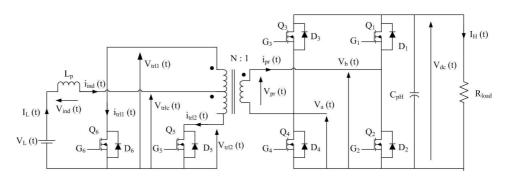
Figure 6-14: Test set-up used to test the operation of the step-up mode of the bidirectional dc-dc converter
