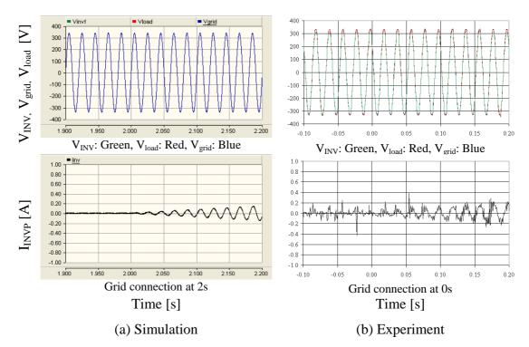
Figure 8-23: Load voltage and inverter output current at the point of grid connection
