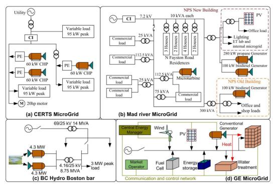
Figure 2-2: Structures of some selected MicroGrids in America
