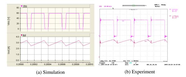
Y axis : V<sub>trlc</sub> – Pink (20V/div), I<sub>ind</sub> – Light brown (1A/div); X axis: Time (10µs/div) Figure C-16: Voltage across the centre of the secondary windings and current flowing through the inductor of the bi-directional dc-dc converter (step-down mode)
