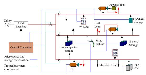
Figure 2-1: Structure of a typical MicroGrid
