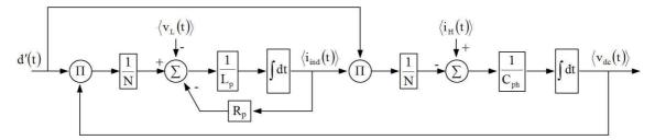
Figure 4-10: State feedback block diagram of the bi-directional dc-dc converter in stepup mode based on the averaged state equations
