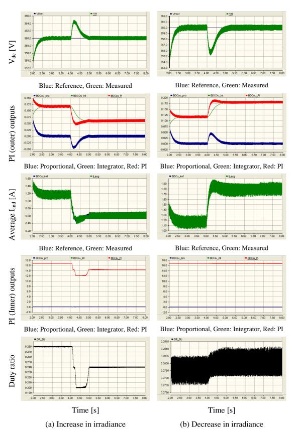
Figure 9-7: Behaviour of the step-up mode controller of the bi-directional dc-dc
