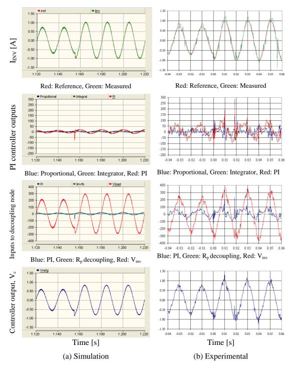
Figure 8-11: Behaviour of the current controller at the step change current reference
