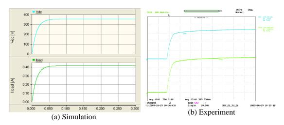
Figure 6-16: Load voltage and load current of the bi-directional converter (step-up
