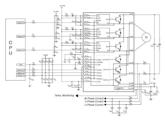
Figure C-17: Typical application diagram of the three-phase inverter module
