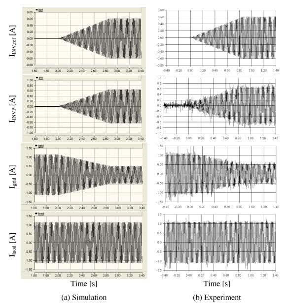
Figure 8-13: Current reference and currents flowing through inverter, load and grid
