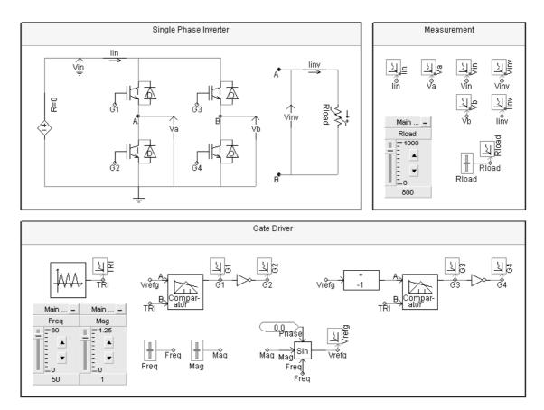
Figure C-24: Screen capture of the simulation model of the single-phase inverter connected to a resistive load
