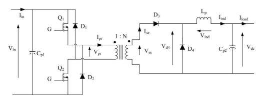
Figure C-1: Schematic diagram of the modified forward dc-dc converter
