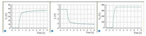
Figure 6-23: Screen capture of the measured waveforms of the bi-directional dc-dc converter (step-down mode) plotted in dSPACE
