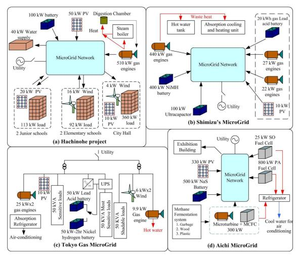
Figure 2-3: Structures of some selected MicroGrids in Japan
