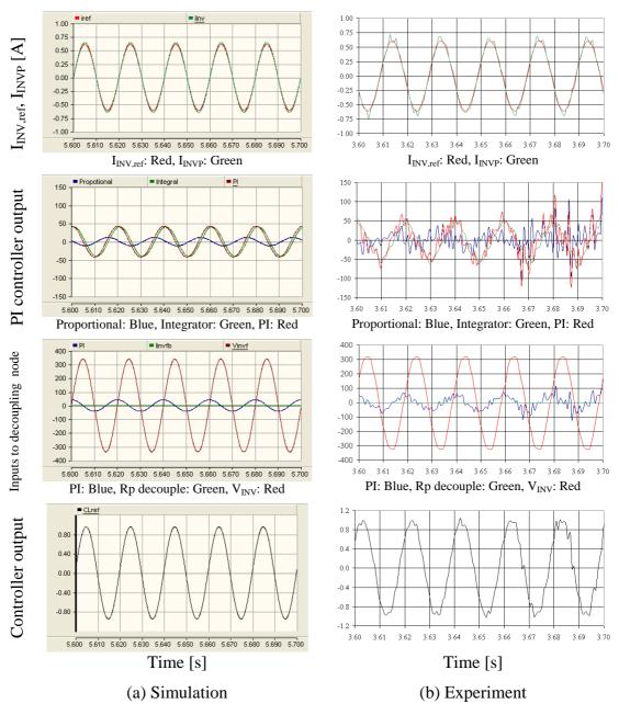
Figure 8-17: Behaviour of current controller of the inverter
