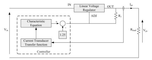
Figure 5-17: Block diagram of the PV Emulator
