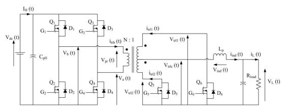
Figure 6-19: Test set-up used to test the operation of the step-down mode of the bidirectional converter
