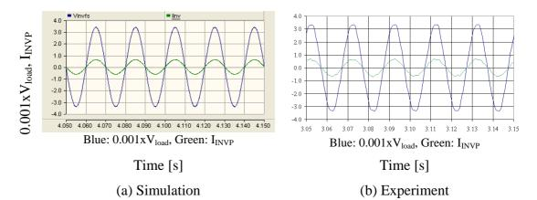
Figure 8-26: Scaled load voltage and inverter output current after the grid connection
