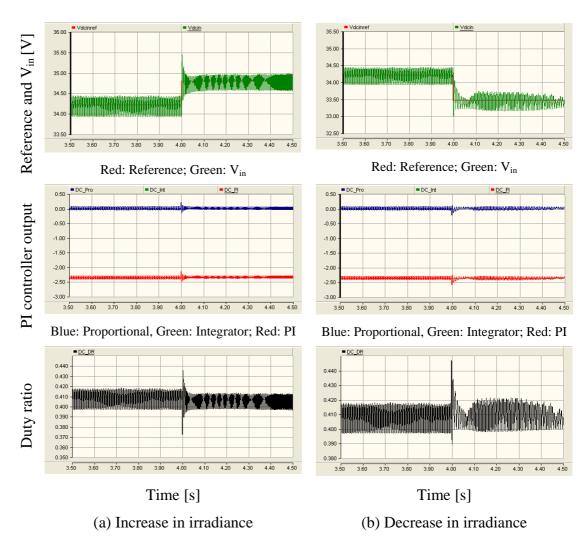
Figure 9-3: Behaviour of the controller of the modified forward dc-dc converter
