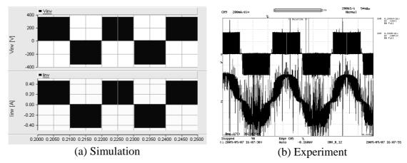
Y axis :Top –  $E_{INV}$  (200V/div), Bottom –  $I_{INV}$  (0.2A/div); X axis: Time (5ms/div) Figure C-26: Voltage across the load and current flowing through the load
