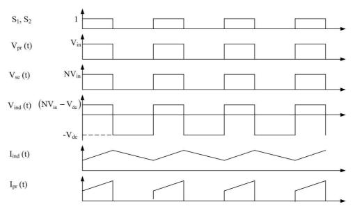
Figure 4-3: Principle of operation of the modified forward dc-dc converter
