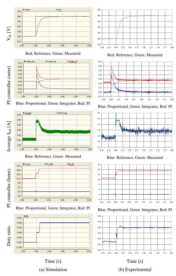
Figure D-24: Behaviour of the controller of the bi-directional dc-dc converter (step-up
