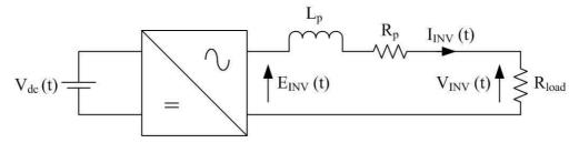
Figure 8-9: Test set-up used for the current controller of the inverter testing
