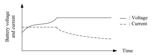
Figure A-5: Voltage and current variation of a battery during constant voltage charging
