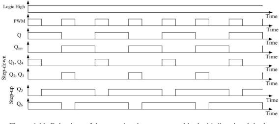
Figure 6-11: Behaviour of the gate signal extractor used in the bi-directional dc-dc converter
