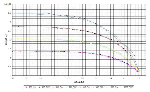
Figure 5-24: Comparison of characteristic curves obtained from simulation model and photovoltaic emulator
