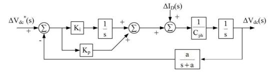
Figure 7-6: Simplified state feedback block diagram of the outer voltage loop of the bidirectional dc-dc converter
