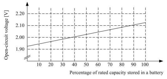
Figure A-4: Variation of open circuit voltage with energy storage in a battery
