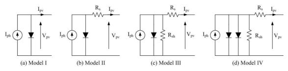
Figure 3-3: Electrical models of a photovoltaic cell
