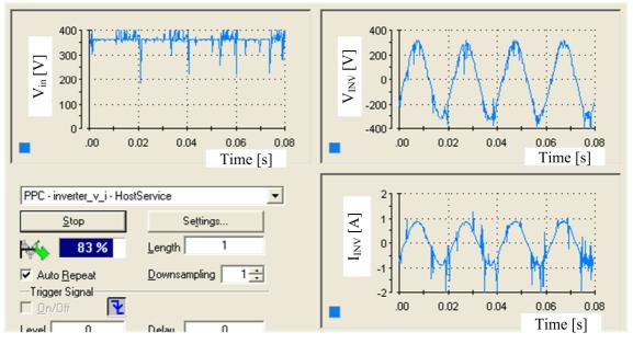
Figure 6-30: Screen capture of the measured quantities of the single-phase inverter plotted in dSPACE
