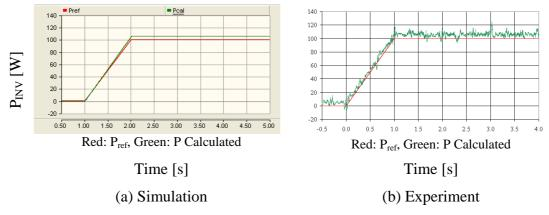
Figure 8-25: Reference and calculated active power of inverter
