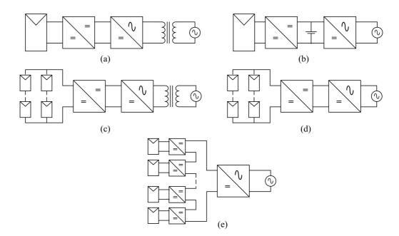
Figure 3-9: Grid connected PV systems with multiple power electronic converters
