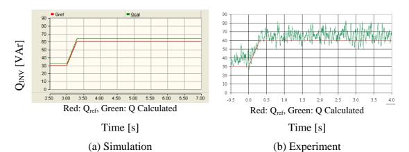
Figure 8-33: Reference and calculated reactive power variation of the inverter
