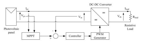
Figure D-2: Structure of the controller used for the modified forward dc-dc converter
