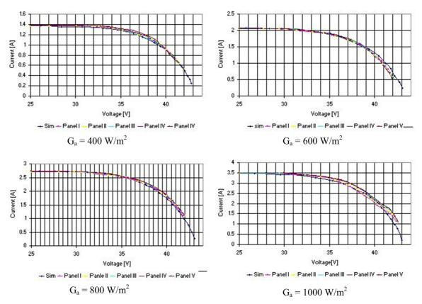
Figure 5-26: Comparison of photovoltaic panels results of simulation model and photovoltaic emulator
