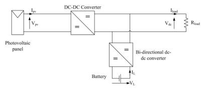
Figure 7-8: Test set-up used to analyse the behaviour of Section-A of the proposed microsource interface
