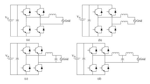
Figure 4-15: Coupling methods used to connect an inverter to a grid
