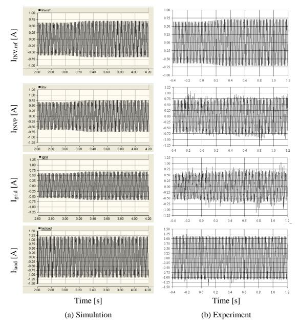
Figure 8-34: Inverter current reference and currents flowing through inverter, grid and
