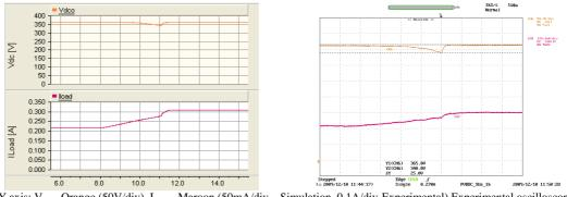
Y axis: V<sub>dc</sub> – Orange (50V/div), I<sub>load</sub> – Maroon (50mA/div – Simulation, 0.1A/div-Experimental) Experimental oscilloscope channel bandwidth = 5kHz; X axis: Time (1s/div)
