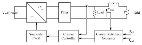
Figure 8-1: Proposed controller for the single-phase inverter
