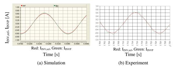
Figure 8-20: Inverter current reference and inverter output current
