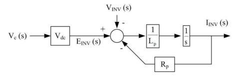
Figure 8-3: State feedback block diagram of the single-phase inverter
