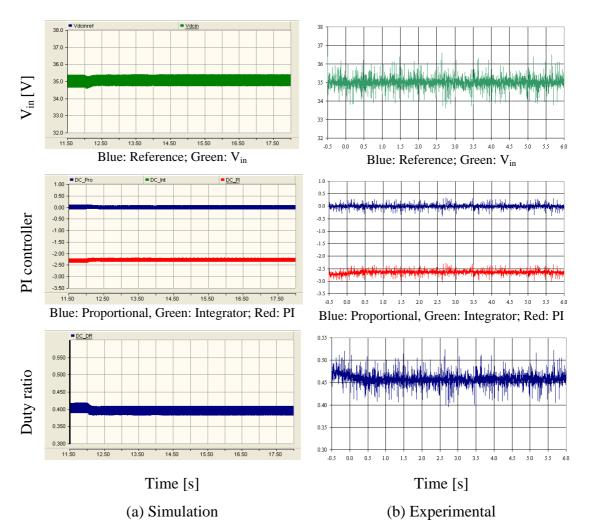
Figure D-44: Behaviour of the controller of the modified forward dc-dc converter
