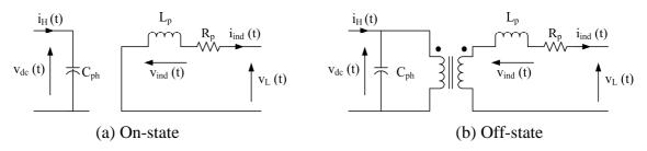
Figure 4-9: Equivalent circuits of the bi-directional dc-dc converter in step-up mode
