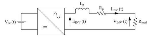
Figure 8-2: Single-phase inverter connected to a series resistive and inductive load
