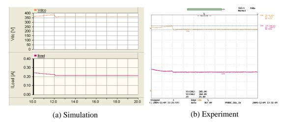
Y axis: V<sub>dc</sub> – Orange (50V/div), I<sub>load</sub> – Maroon (0.1A/div) Experimental oscilloscope channel bandwidth = 5kHz, In the experimental results ground level is same for both channels; X axis: Time (1s/div) Figure 7-9: DC-link voltage and load current (Automatic step-down mode turn-on
