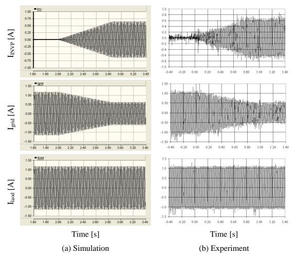
Figure 8-22: Current flowing through the grid, load and inverter
