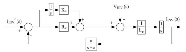
Figure 8-5: Simplified current controller for the single-phase inverter
