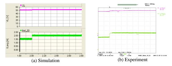
Y axis:  $V_L$  – Pink (10V/div),  $I_L$  – Light green (0.5A/div); X axis: Time (100ms/div) Figure D-36: Voltage at the low-voltage end of the bi-directional dc-dc converter and the battery current
