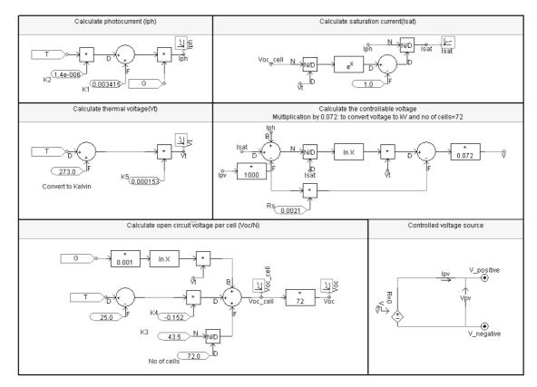
Figure B-3: Screen capture of the simulation model of the photovoltaic panel purely based on the characteristic curve
