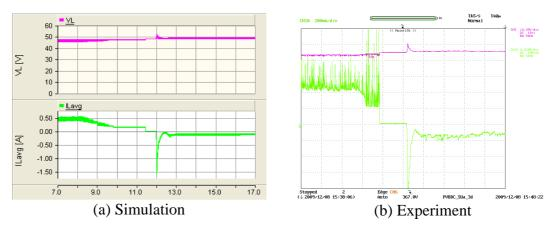
$\label{eq:VL} \begin{array}{l} Y \mbox{ axis: } V_L - Pink \mbox{ (10V/div), } I_L - Green \mbox{ (Simulation-0.5A/div, Experiment-0.2A/div), } For experimental measurements} \\ \mbox{ oscilloscope channels bandwidth} = 5 kHz; X \mbox{ axis: Time (1s/div)} \end{array}$
