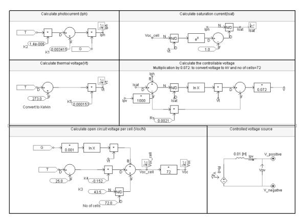
Figure B-4: Screen capture of the simulation model of the photovoltaic panel with inductor in series with voltage source
