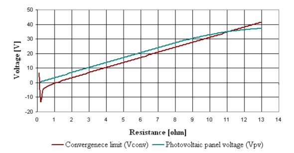
Figure 5-8: Variation of convergence limit  $(V_{conv})$  and photovoltaic panel voltage  $(V_{pv})$ with load resistance (R)
