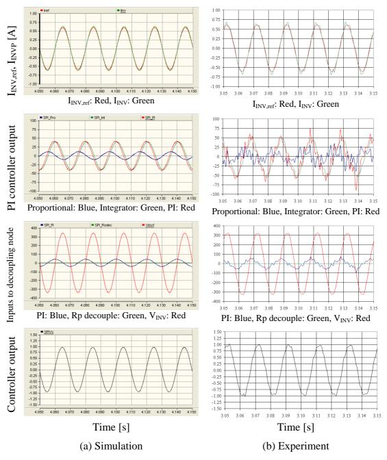
Figure 8-30: Behaviour of the controller of the current controller
