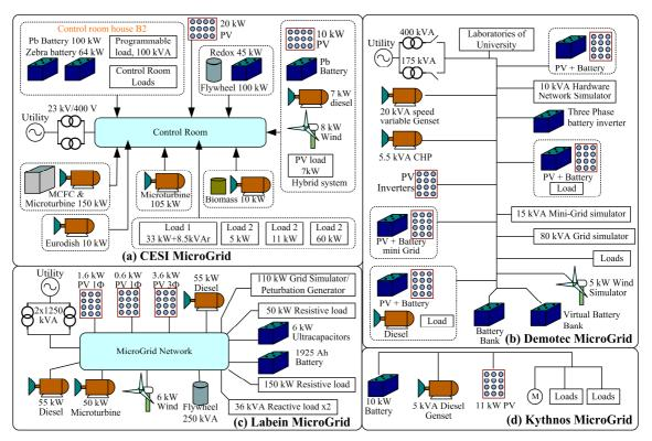
Figure 2-4: Structures of some selected MicroGrids in Europe
