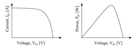
Figure 3-2: Characteristic curves of a photovoltaic cell
