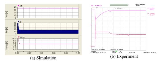
Y axis : $V_{in}$  - Pink (10V/div, top),  $I_{in}$  – Maroon (2A/div, bottom) ; X axis: Time (100ms/div) Figure 6-4: Input voltage and input current of the modified forward dc-dc converter
