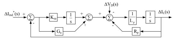
Figure 7-5: Simplified state feedback block diagram of the inner current loop of the bidirectional dc-dc converter
