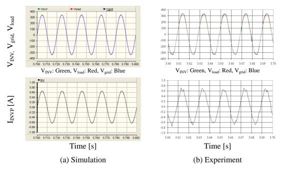
Figure 8-15: Load voltage and inverter output current after grid connection
