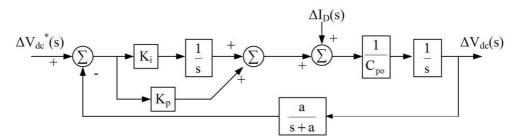
Figure D-38: Simplified outer voltage control loop
