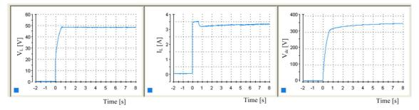
Figure 6-18: Screen capture of the measured waveforms of the bi-directional converter (step-up mode) plotted in dSPACE
