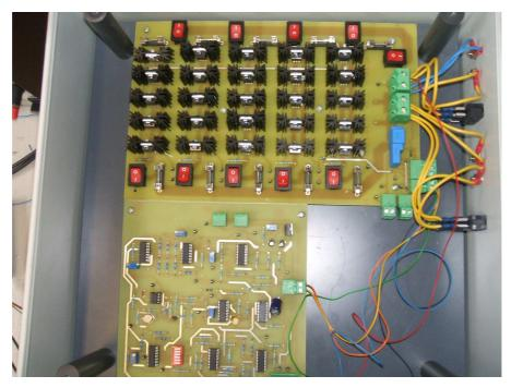
Figure 5-27: Picture of the photovoltaic emulator
