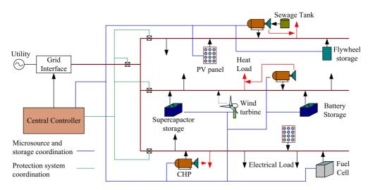
Figure 1-1: Structure of a typical MicroGrid
