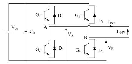
Figure C-18: Single-phase inverter under open circuit test
