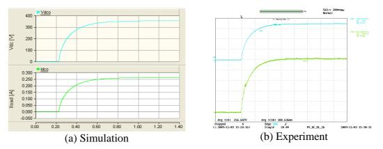
Y axis:  $V_{dc}$  – Light blue (100V/div),  $I_{load}$  – Light green (50mA/div) Experimental oscilloscope channel bandwidth = 5kHz; X axis: Time (200ms/div)
