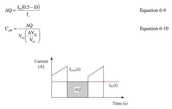
Figure 6-9: Input and output current through the high side capacitor node of the bidirectional dc-dc converter
