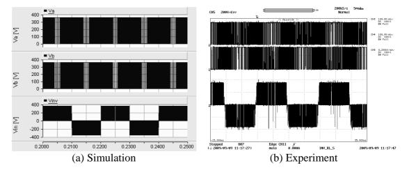
Y axis : Top - V<sub>A</sub> (100V/div-simulation, 200V/div-Experiment), Middle –V<sub>B</sub> (100V/div-Simulation, 200V/div-Experiment), Bottom – E<sub>INV</sub> (200V/div); X axis: Time (5ms/div)
