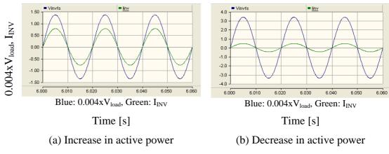
Figure 9-10: Scaled load voltage and inverter output current
