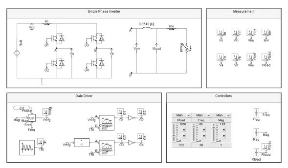
Figure C-30: Screen capture of the simulation model of the single-phase inverter connected to a RL load
