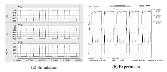
$\label{eq:constraint} \begin{array}{l} Y \mbox{ axis :} Top-G_3 \mbox{ (2V/div-Experiment), Middle} - G_4 \mbox{ (2V/div-Experiment), Bottom} - V_B \mbox{ (100V/div-Simulation, 200V/div-Experiment); X \mbox{ axis: Time (50 $\mu$s/div)} \end{array}$
