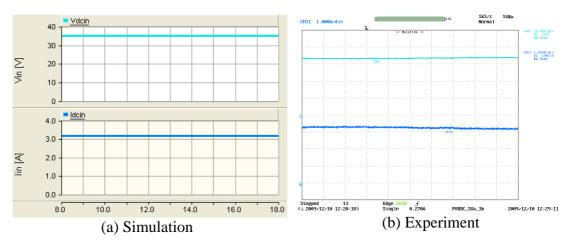
Y axis:  $V_{in}$  – Light blue (10V/div),  $I_{pv}$  – Dark blue (1A/div), For experimental results oscilloscope channel bandwidth = 5kHz,; X axis: Time (1s/div)
