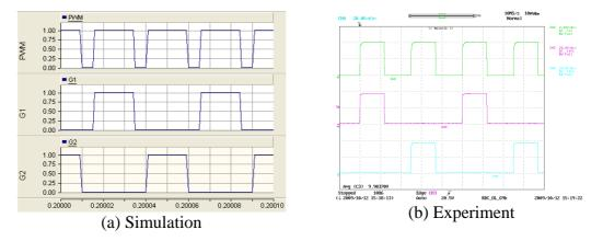
Y axis : Simulations- [Top: PWM, Middle: (Q<sub>1</sub>, Q<sub>4</sub>), Bottom: (Q<sub>2</sub>, Q<sub>3</sub>)], Experiment – [Top: PWM - Green (2V/div), Middle: (Q<sub>1</sub>, Q<sub>4</sub>) - Pink (2V/div), Bottom: (Q<sub>2</sub>, Q<sub>3</sub>) - Blue (2V/div)] ; X axis: Time (10µs/div) Figure 6-12: Gate signals during step-down mode of the bi-directional dc-dc converter
