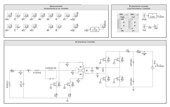
Figure C-12: Screen capture of the simulation model of the bi-directional dc-dc converter operating in step-down mode
