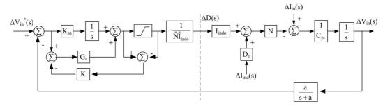
Figure D-8: Controller of the modified forward dc-dc converter with an integrator antiwind up block
