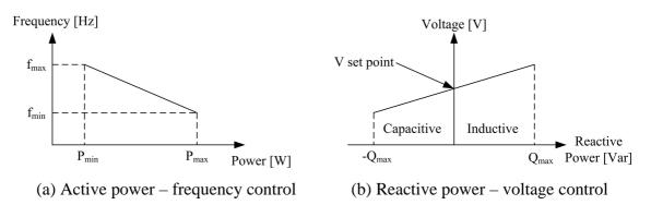
Figure 2-7: Active and reactive power control of a microsource
