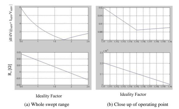
Figure 5-3: Variations of absolute difference and series resistance with ideality factor
