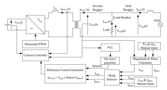
Figure 8-12: Detailed controller of the single-phase inverter
