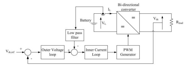
Figure 7-4: Controller of the bi-directional dc-dc converter
