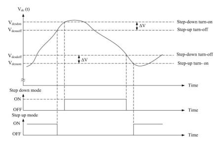
Figure 7-7: Hysteresis control technique used to control the operating modes of the bidirectional dc-dc converter
