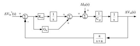
Figure 7-3: Simplified state feedback block diagram of the controller of the modified forward dc-dc converter
