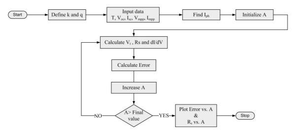
Figure 3-6: Algorithm used to find ideality factor and the series resistance
