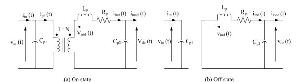
Figure 4-4: Equivalent circuit of the modified forward dc-dc converter
