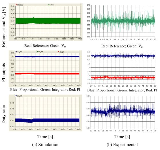
Figure 7-17: Behaviour of the controller of modified forward dc-dc converter (Automatic step-up mode turn-on transient)
