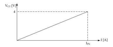
Figure 5-19: Characteristic curve of the current transducer
