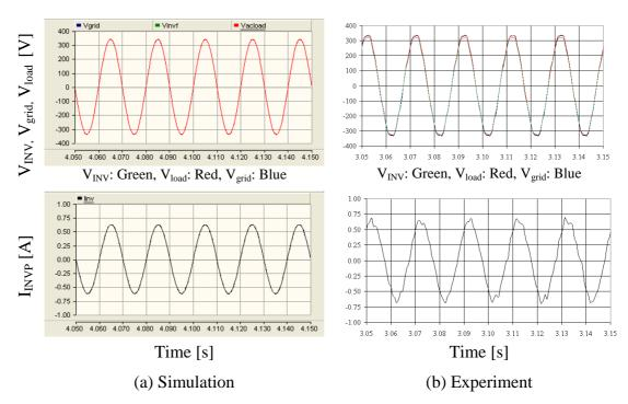
Figure 8-29: Voltages and inverter output current after grid connection
