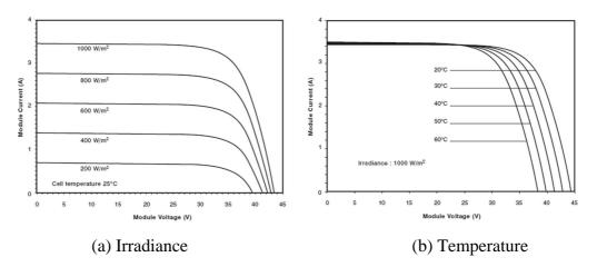
Figure 3-4: Effect of environmental conditions on characteristic curves
