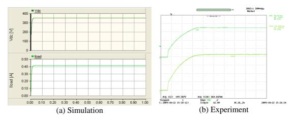
Y axis :V<sub>dc</sub> – Dark green (100V/div),  $I_{load}$  – Light green (100mA/div), Exp. Scope bandwidth 5kHz ; X axis: Time (100ms/div)
