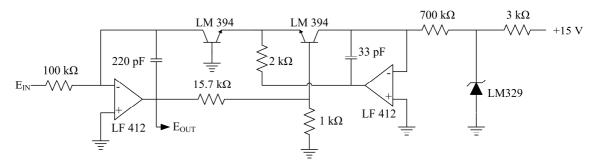
Figure 5-20: Schematic diagram of a logarithmic amplifier
