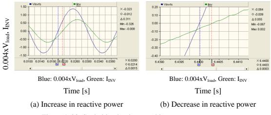
Figure 9-20: Scaled load voltage and inverter output current
