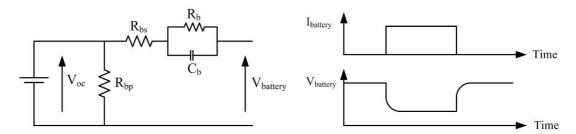
Figure A-8: Thevenin's equivalent circuit of a battery
