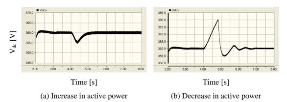
Figure 9-13: Variation of dc-link voltage
