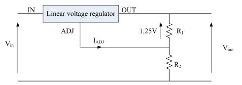
Figure 5-14: Typical application diagram of an adjustable linear voltage regulator
