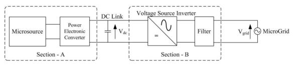
Figure 2-5: Simplified model of a microsource interface
