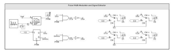
Figure C-7: PWM generator and signal extractor used to test the step-up mode
