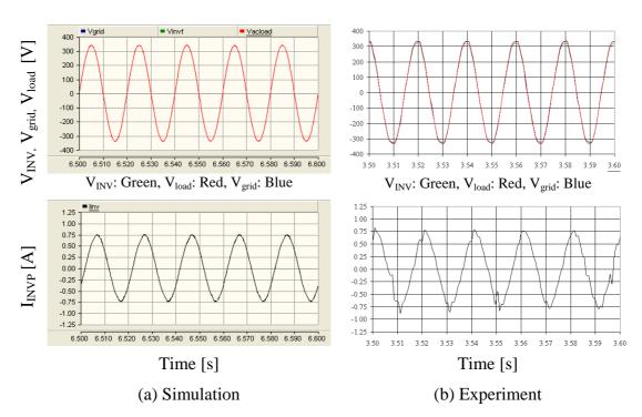
Figure 8-36: Voltages and current after the increase of the reactive power reference
