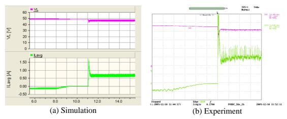
Y axis:  $V_L$  – Pink (10V/div) Experimental oscilloscope channel bandwidth = 5kHz,  $I_L$  – Green (0.5A/div – Simulations, 0.2A/div-Experimental); X axis: Time (100ms/div)
