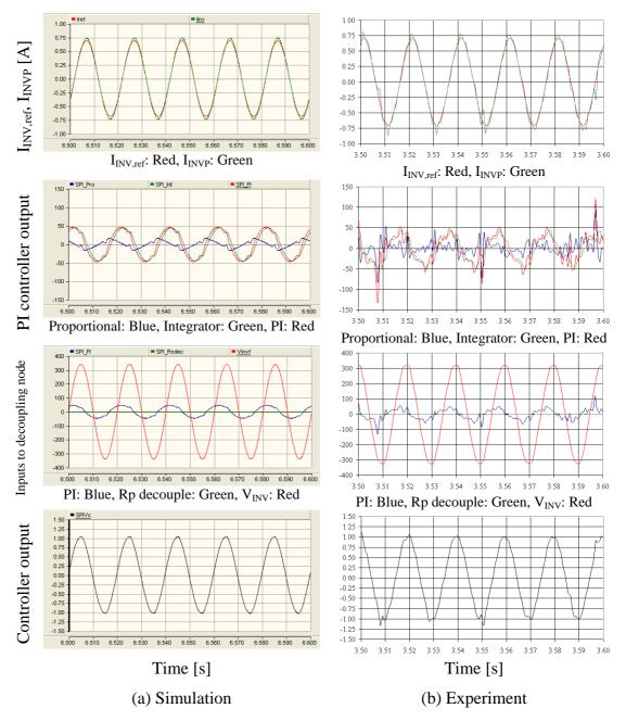
Figure 8-37: Behaviour of the current controller
