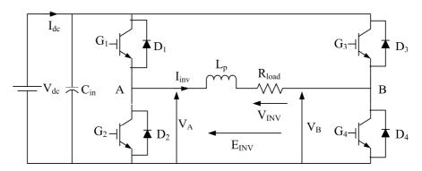
Figure 6-25: Single-phase inverter connected to a series inductive and resistive load
