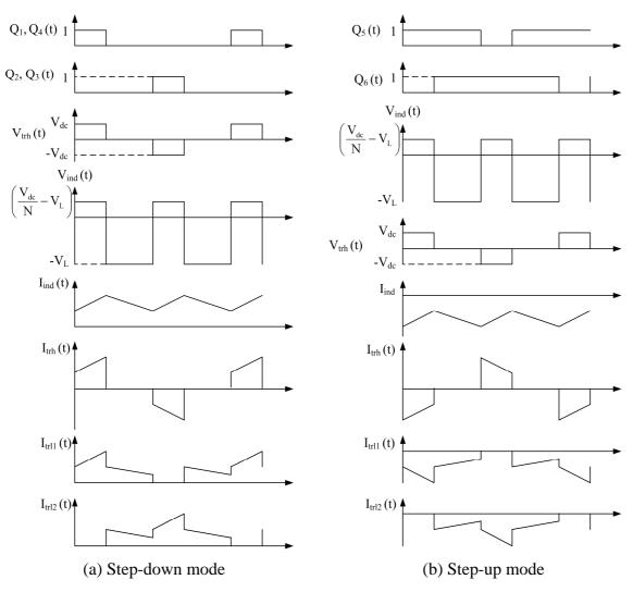
Figure 4-8: Principle of operation of the bi-directional dc-dc converter
