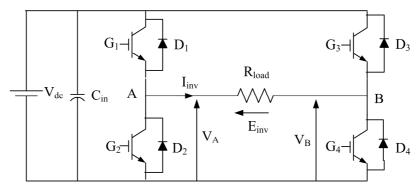
Figure C-23: Single-phase inverter connected to a resistive load
