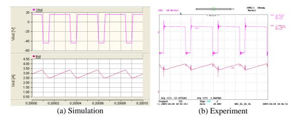
Y axis :V<sub>ind</sub> – Pink (20V/div), I<sub>ind</sub> – Maroon (simulation: 0.5A/div, Experiment: 1A/div); X axis: Time (10µs/div) Figure 6-22: Voltage across the inductor and current flowing through the inductor of the bi-directional dc-dc converter (step-down mode)
