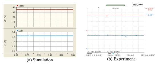
Y axis: V<sub>dcin</sub> – Brown (10V/div), I<sub>pv</sub> – Blue (1.0A/div), Experimental results oscilloscope channel bandwidth = 5kHz; X axis: Time (100ms/div)
