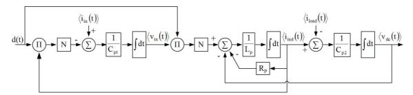
Figure 4-5: State feedback block diagram of the modified forward dc-dc converter based on averaged state equations
