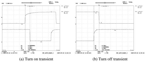
Y axis :Top –  $\overline{G}_1$  (2V/div), Bottom –  $\overline{G}_2$  (2V/div); X axis: Time (5µs/div) Figure 6-24: Gate signals applied to an arm of the single-phase inverter module
