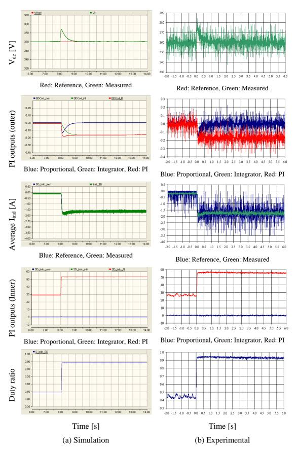
Figure 7-37: Behaviour of the step-down mode controller of the bi-directional dc-dc converter (Step-down mode worst-case)
