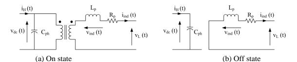
Figure 4-12: Equivalent circuits of the bi-directional dc-dc converter in step-down mode
