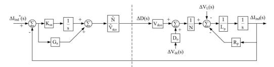
Figure D-33: Block diagram of the inner current control loop of the bi-directional dc-dc converter (step-down mode)
