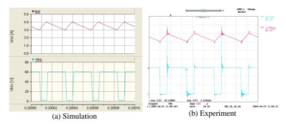
Y axis :I<sub>L</sub> – Light brown (1A/div), V<sub>trlc</sub> – Light blue (20V/div) ; X axis: Time (10µs/div) Figure C-8: Voltage at the centre of the transformer and current flowing through the inductor of the bi-directional converter (step-up mode)
