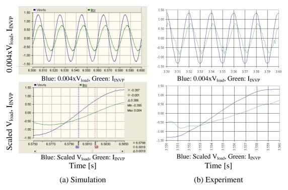
Figure 8-38: Scaled load voltage and inverter output current after the increase of current reference
