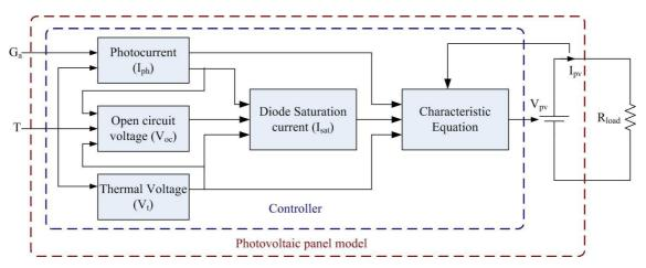
Figure 5-4: Block diagram of the simulation model of the photovoltaic panel
