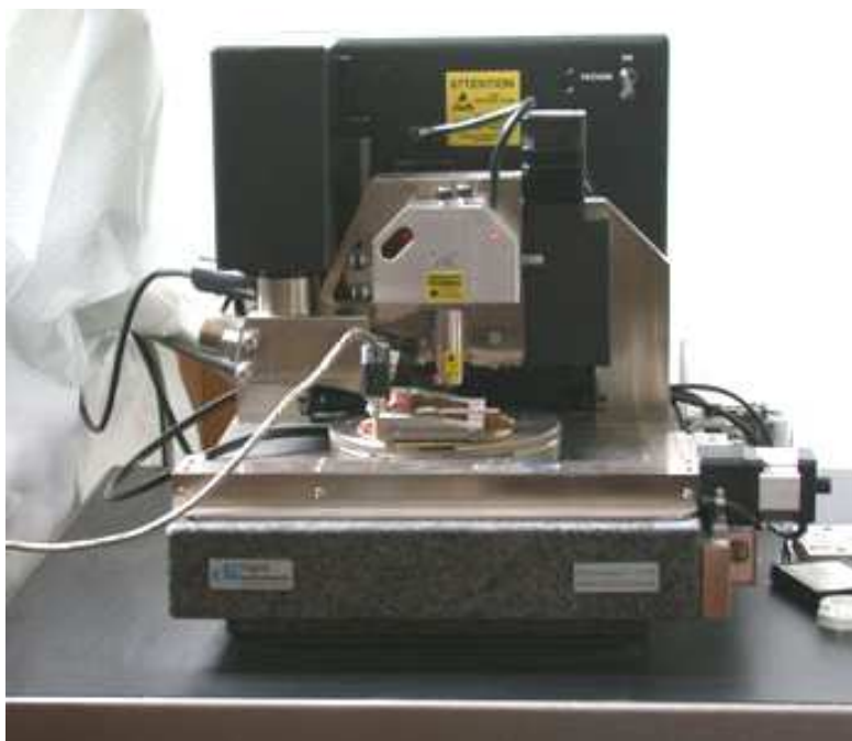
Figure 3.8 Image of Veeco CP2 atomic force microscope
