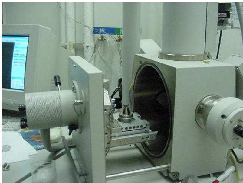
Figure 3.7 Philips XL30 ESEM-FEG scanning electron microscope.
