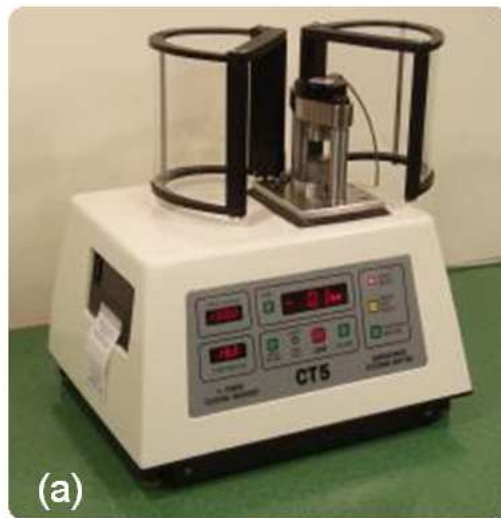
Figure 3.2 Picture of surface micro-cracks testing machine, employed for optic grating press over aluminium substrate.
